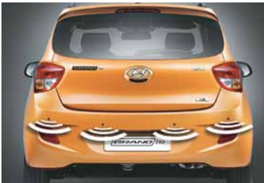
REAR PARKING SENSOR Useful for parking in tight spaces and detect obstructions while reversing
