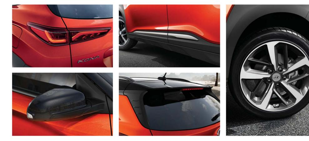
LED rear lamps Two-tone exterior mirrors with LED indicator Sporty silver side sill Two-tone roof and rear spoiler 18" alloy wheels
