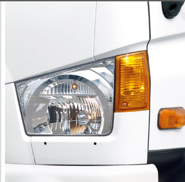
MFR Headlamps (Multi Focus Reflection)
