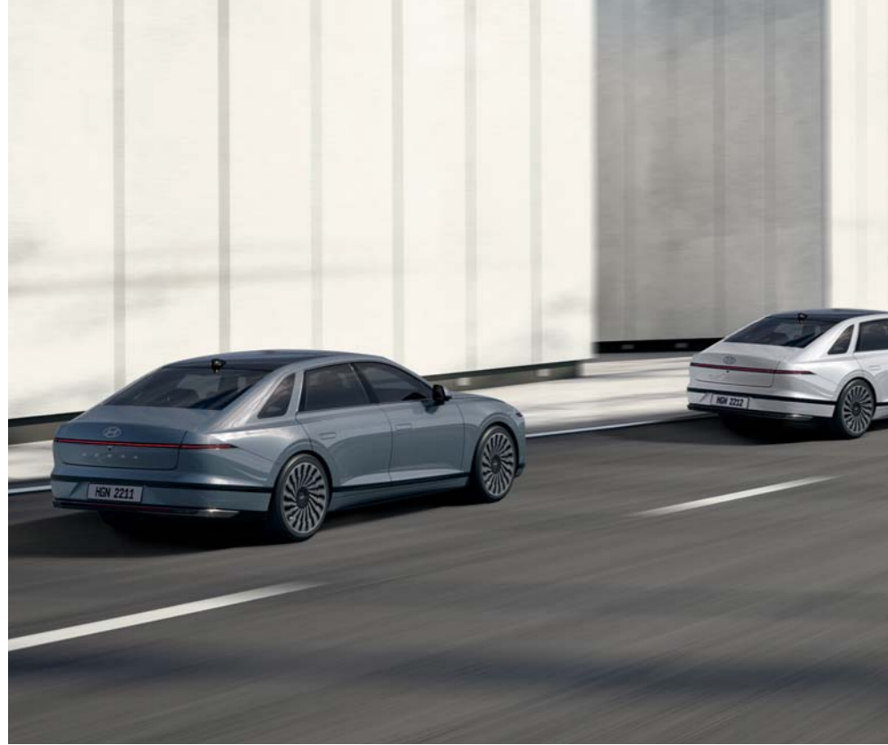
Smart Cruise Control (SCC) Smart Cruise Control (SCC) helps maintain distance from the front vehicle and drive at a speed set by the driver. Automatically stops when the front vehicle stops and starts automatically when the front vehicle departs within a short time.
