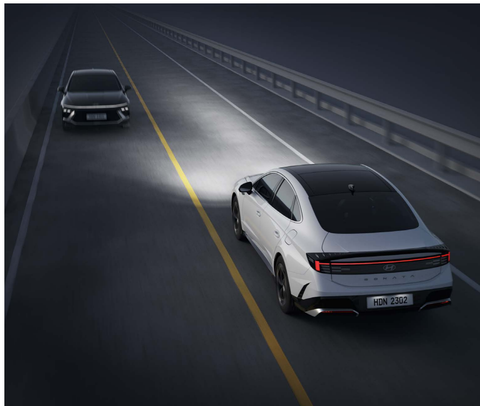
High Beam Assist (HBA) High Beam Assist (HBA) automatically adjusts the high beams by detecting ambient light and illuminance, such as a lamp of an oncoming vehicle or a preceding vehicle.
