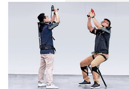
VEX – vest-type wearable robot; and CEX – chair-type industrial exoskeleton robotic system
