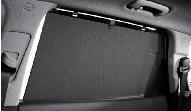
Rear window sunshades 2 A retractable window blind hidden away in the 2nd row doors protect your precious ones from the heat and glare of the summer sun.
