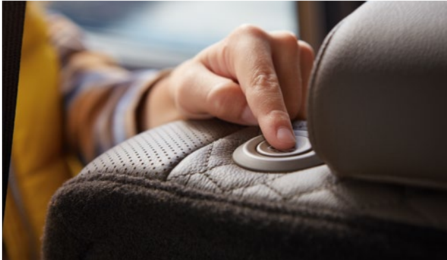
Smart one-touch walk-in 1 Collapse and slide forward the seats in the 2nd row at the touch of a button, giving easy access for kids getting in and out of the 3rd row.
