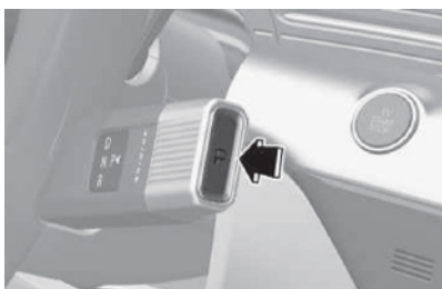
Step on brake pedal to park the vehicle, then position the shift lever in Park (P)
