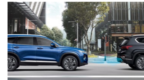
Smart Cruise Control (SCC) with Stop & Go Detects the speed and distance of vehicles ahead of the Santa Fe and maintains a safe distance to the vehicle ahead, up to a pre-set speed (between 30km/h – 160km/h). The Stop & Go function works in stop/start traffic, bringing the vehicle to a stop when appropriate, and automatically (if within 3 seconds) accelerate back up to the original set speed.
