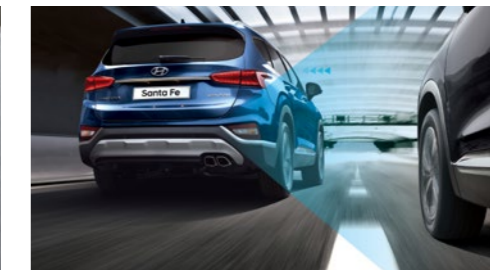
Blind-Spot Collision-Avoidance Assist (BCA) Blind-Spot Collision-Warning will send visual warnings to the driver when a vehicle is in their blind spot and an audible sound if the driver tries to change lanes with the vehicle still in their blind spot. Blind-Spot Collision-Avoidance Assist will initiate an active avoidance manoeuvre if necessary to avoid potential accidents.
