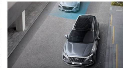
Safe Exit Assist (SEA) 3 The system detects any oncoming vehicles approaching from the rear and alerts the driver that it may be dangerous for passengers to exit the vehicle, with both a sound and pop-up visual warning on the dashboard. If the child safety lock is activated, the SEA system will prevent the door from being unlocked to prevent opening.
