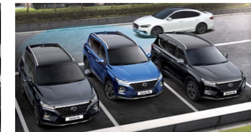
Rear Cross-Traffic Collision-Avoidance Assist (RCCA) When backing out from a parking position, the sensor detects approaching vehicles from the left or right. The sensor will issue an audible alert and visual warning on the dashboard and if necessary, will initiate a braking manoeuvre.
