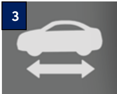
3 The 'Ready' light indicates the vehicle is 'ON' and ready for driving.
