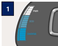
1 Regeneration Brake/ECO/Power Gauge
