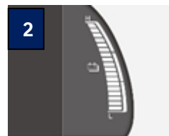
2 SOC (High Voltage battery). The gauge indicates the charge state of the high voltage battery.
