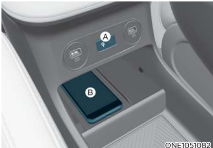
[A] : Indicator light, [B] : Charging pad
