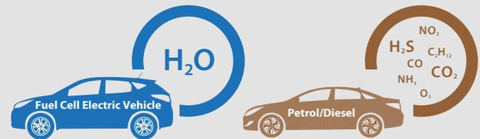
A Fuel Cell Electric Vehicle does not burn Hydrogen, instead a chemical reaction between Hydrogen and Oxygen creates electricity to drive a motor. No harmful pollutants are emitted.
