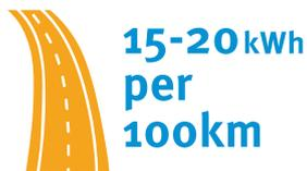
This means that the average EV uses 15-20 kWh for every 100km.
