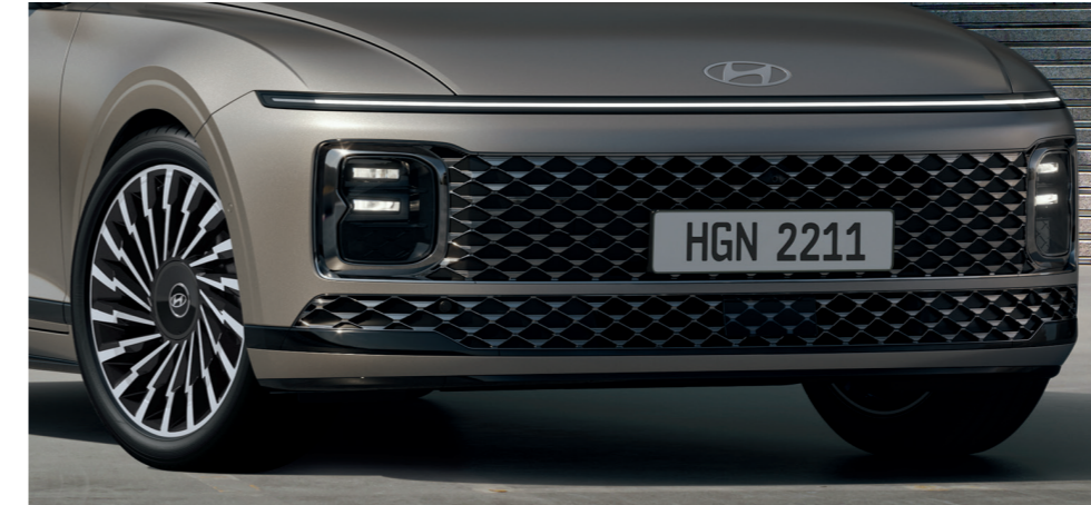
Parametric Pattern Grille / Horizontal LED lamp (Seamless Horizon Lamp) / Full LED Headlights (Projection Type)
