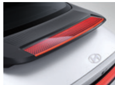
Parametric pixel high-mounted stop lamp (HMSEL)
