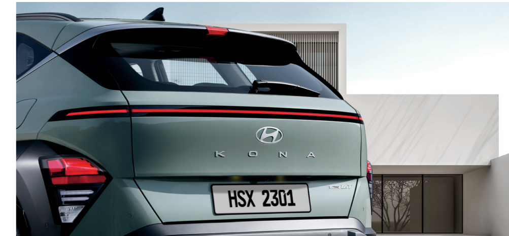
Spoiler Integrated HMSL, rear seamless horizon lamp, LED brake lamps, LED turn signal lamps
