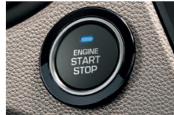
**Smart key & engine Start/Stop button.** Keyless starting when the smart key is on board in your pocket or bag.
