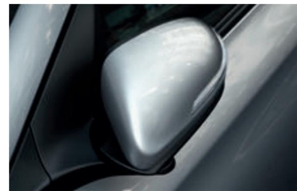
**Power folding door mirrors.** The door mirrors can be electrically folded against the body. Useful when parked in tight spaces.
