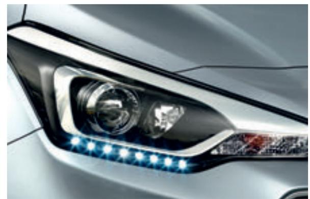
**High performance projector headlamps.** Combined with LED daytime running lights and static cornering lights.
