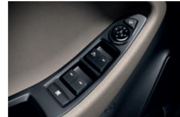
**Electric windows in all doors.** The driver's window has a one-touch Auto up/down function with anti-trap feature.
