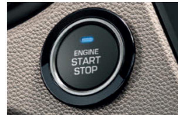
**Smart key & engine Start/Stop button.** Keyless starting when the smart key is on board in your pocket or bag.
