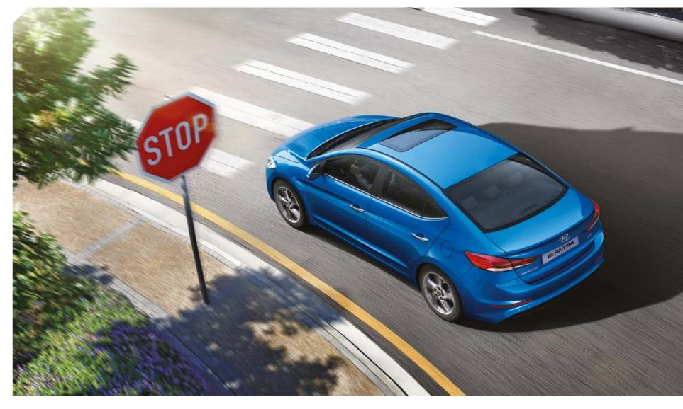
**ELECTRONIC STABILITY CONTROL (ESC)** Electronic stability control detects and reduces loss of traction during sudden braking and turning movements. Using automatic braking for individual wheels and reducing engine power helps a vehicle to maintain stability and control.
