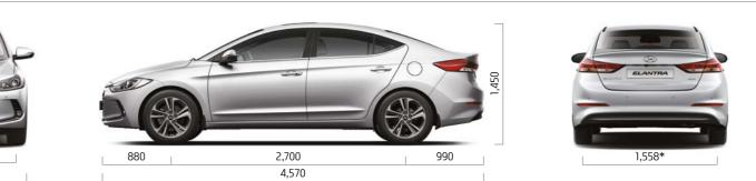
\* Wheel tread •15" alloy wheels (Front/rear): 1,563/1,572 •16" alloy wheels (Front/rear): 1,555/1,564 •17" alloy wheels (Front/rear): 1,549/1,558
