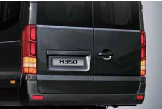
Under heavy emergency braking, the hazard warning lights are automatically activated
