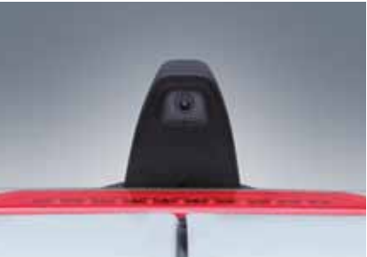
Rear camera feeds visual information to the in-cab display
