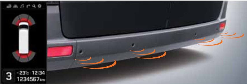
Park Assist System (PAS) uses strategically positioned sensors, front and rear, to detect potential obstructions when parking
