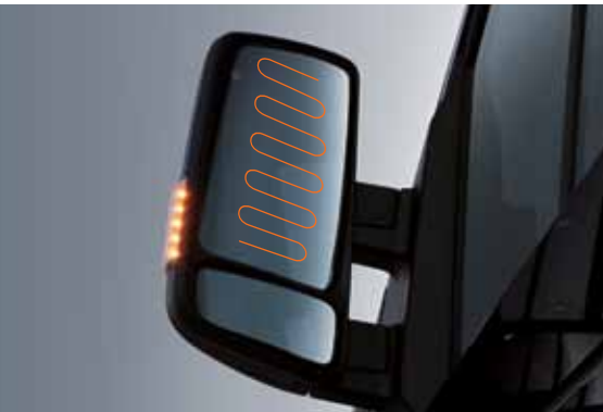
Side mirrors are electrically adjusted and heated
