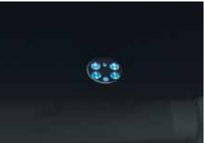
Rain sensors activate windscreen wipers when necessary
