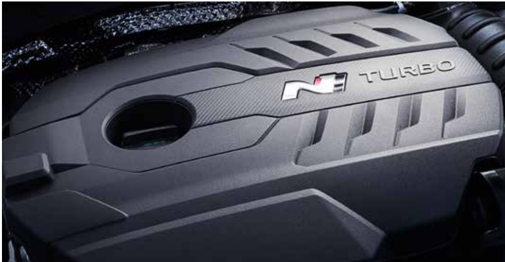
The 2.0 Direct Injection Turbo engine delivers a choice of 250 HP in the Standard Package, or 275 HP in the Performance Package. Both variants generate a maximum torque of 353 Nm.
