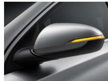
LED outside mirror repeaters LED 側鏡指揮燈
