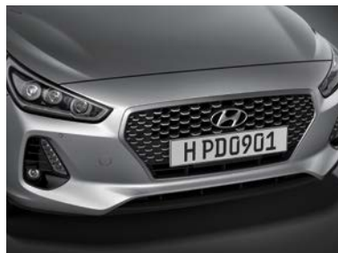
Front parking assist system (FPAS) 前泊車感應器
