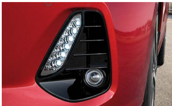
LED daytime running lights (DRL) & fog lamps LED 日間行車燈及霧燈
