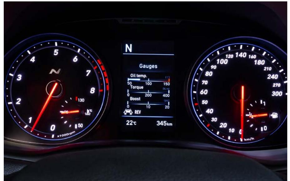
The N instrument cluster is customised for passionate drivers. You can monitor engine oil temperature, torque, and turbo boost at a glance. Featuring a shift timing to support track driving, the red zone of the variable LED rev-counter changes according to engine temperature.
