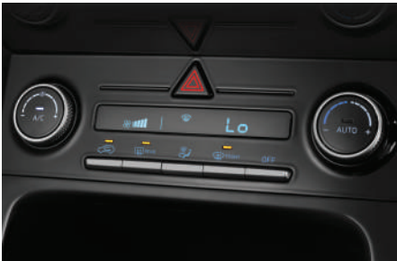
Full Automatic Temperature Controls
