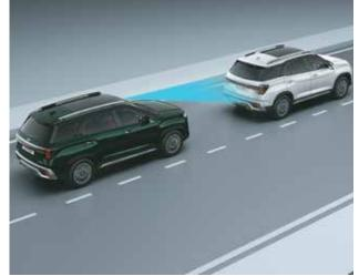
Forward Collision - Avoidance Assist - Car (FCA-Car) & Forward Collision Warning (FCW) - Pedestrian (FCA-Ped)
