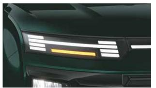
LED turn signal with sequential function
