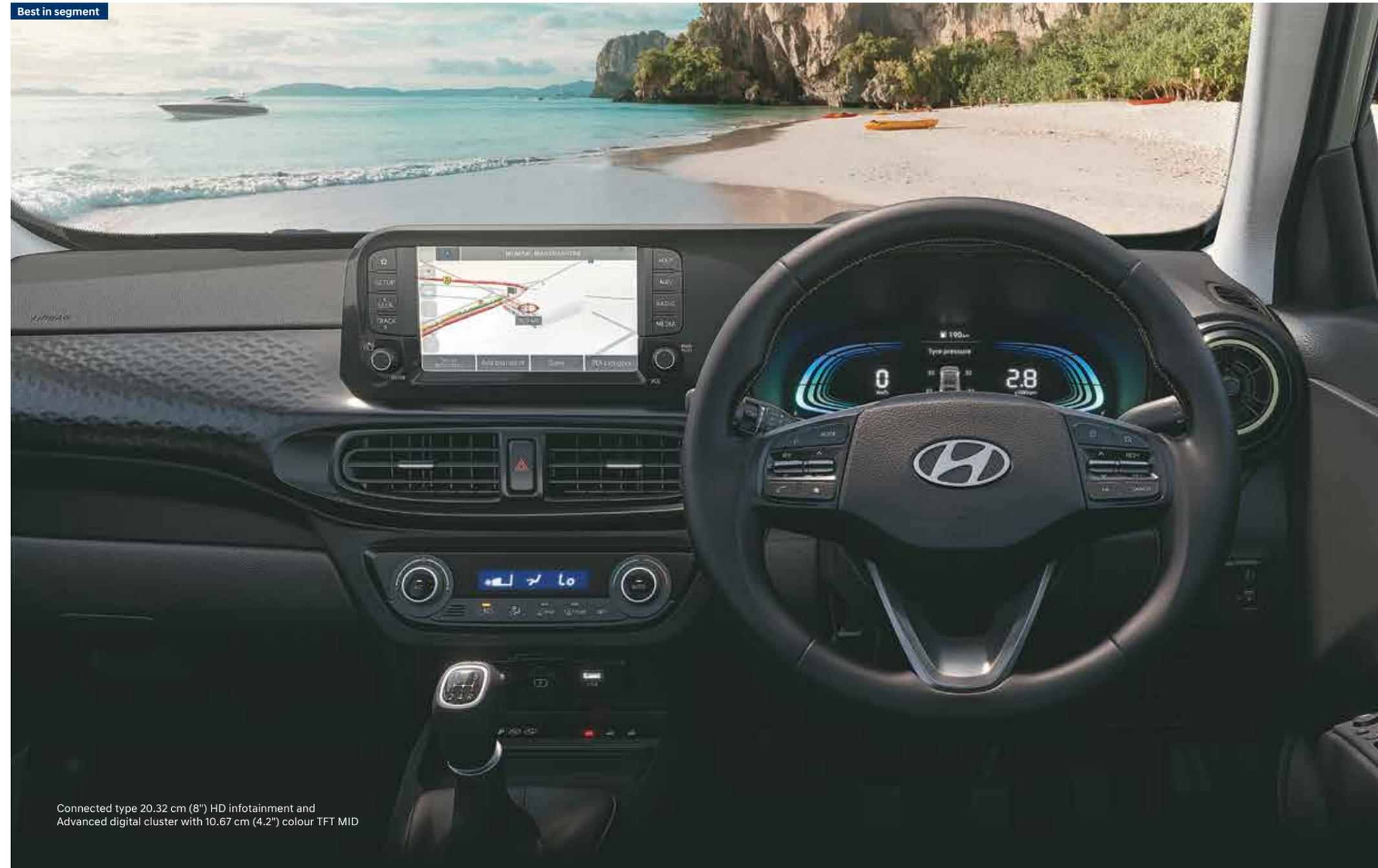
Connected type 20.32 cm (8") HD infotainment and Advanced digital cluster with 10.67 cm (4.2") colour TFT MID
