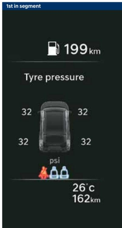
Tyre pressure monitoring system – Highline
