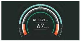
Smart eco pedal guide-encourages fuel efficient driving
