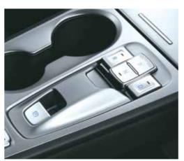
Shift-by-wire automatic transmission and electric parking brake
