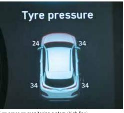
Tyre pressure monitoring system (high line)
