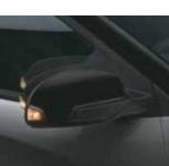
ORVM (heated) with electric adjust and folding
