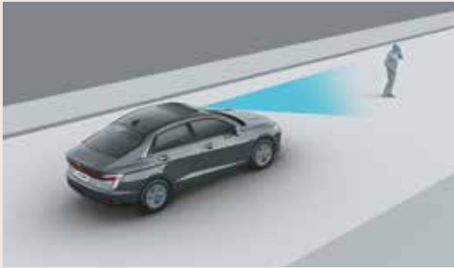
Forward Collision - Avoidance Assist - Pedestrian (FCA-Ped)
