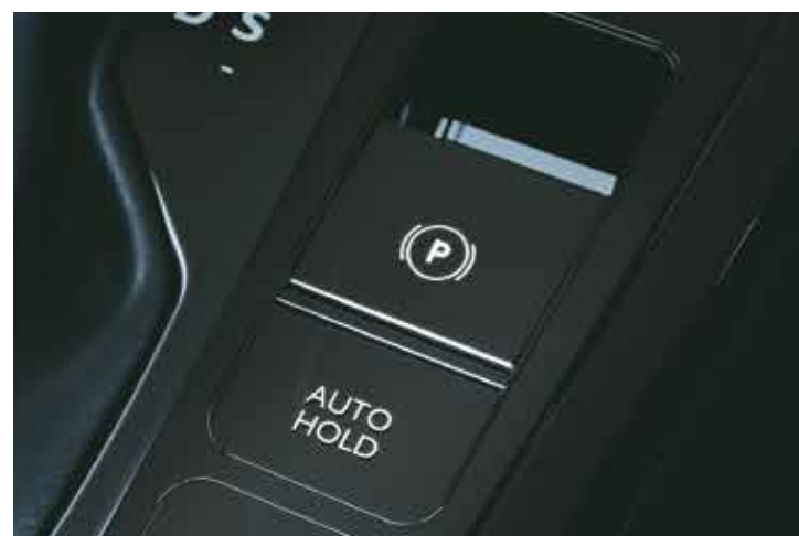
Electric parking brake with auto hold
