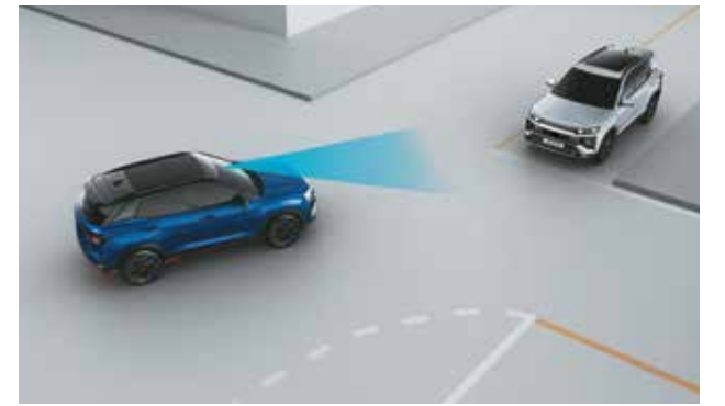
Forward Collision - Avoidance Assist - Junction Turning (FCA-JT) & Forward Collision - Avoidance Assist - Direct Oncoming (FCA-DO)
