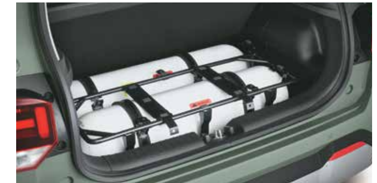
Company fitted dual cylinder CNG
