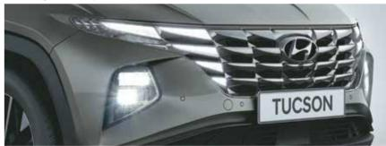
Dark chrome parametric front grille with parametric hidden LED DRLs, LED MFR headlamps & positioning lamps
