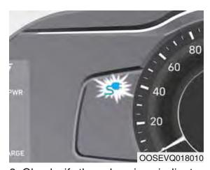
8. Check if the charging indicator light of the high voltage battery in the instrument cluster is turned ON. Charging is not done when the charging indicator lamp is OFF.
