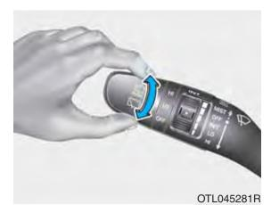
The rear window wiper and washer switch is located at the end of the wiper and washer switch lever.
