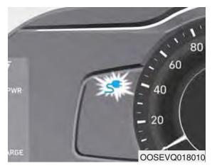
10. Check if the charging indicator light of the high voltage battery in the instrument cluster is turned ON. Charging is not done when the charging indicator lamp is OFF.
