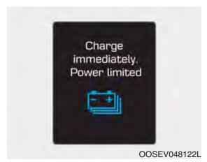
When the high voltage battery level reaches below approximately 3%, this warning message is displayed.
