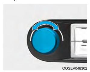
The temperature will increase by turning the knob to the right. The temperature will decrease by turning the knob to the left.
