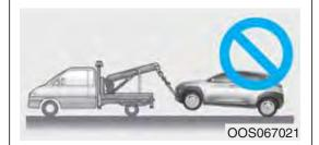
Do not tow with sling-type equipment. Use wheel lift or flatbed equipment.
