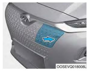
5. Push the charging door where the icon is located to open. The charging door opens only when the door is unlocked.
