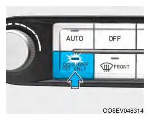
If you press the DRIVER ONLY button( \$\mathbb{G}^{\text{DRIVER}}\_{\text{ONLY}}) and the indicator light illuminates, cold air mostly blows in the direction of the driver's seat. However, some of the cold air may come out of other seating position ducts to keep indoor air pleasant.
