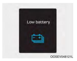
When the high voltage battery level reaches below approximately 8%, this warning message is displayed.
