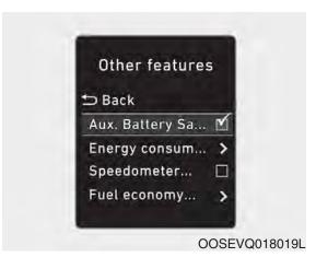
The driver can activate the Aux. Battery Saver+ function by placing the START/STOP button to the ON position and by selecting:
