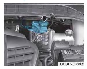
Check the fluid level in the reservoir periodically. The fluid level should be between MAX and MIN marks on the side of the reservoir.
