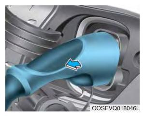
1. Hold the charging connector handle and pull it out.
