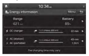
You can check the reachable range, total battery power remaining, and expected charging time for each charge type.
