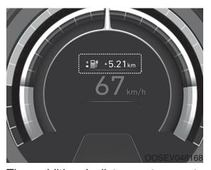
The additional distance to empty which is converted from the energy regenerated by the regenerative braking is displayed if the ECO/ECO+ mode is selected by pressing the Drive Mode button. The display is initialized to 0 if the regenerative braking stops because of acceleration, etc.
