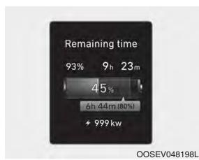
8. After charging has started, the estimated charging time is displayed on the instrument cluster for about 1 minute.
