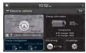
Select 'EV → Charge management' on the screen. You can set the date and time of when to charge the battery, climate control temperature, location-based charging options and other various functions.
