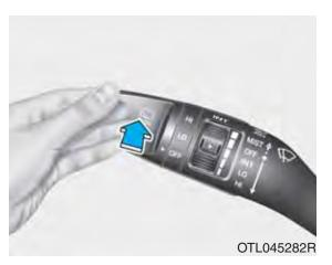
Push the lever away from you to spray rear washer fluid and to run the rear wipers 1~3 cycles. The spray and wiper operation will continue until you release the lever (if equipped).
