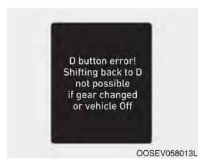
The message is displayed when there is a problem with the D button. If this message is displayed, do not shift the gear or turn the vehicle off while driving. If the driver shifts the gear to P/R/N position or turns off the engine, it is impossible to shift back to D (Drive).
