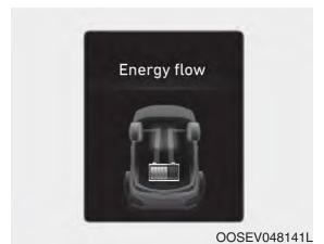
The high-voltage battery is charged up by the regenerative brake system.
