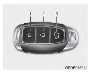
Your HYUNDAI uses a Smart Key, which you can use to lock or unlock a door (and tailgate) and even start the vehicle.
