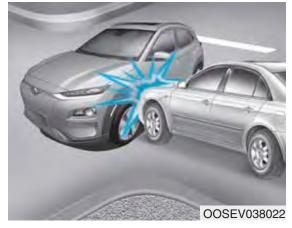
Front air bags may not inflate in side impact collisions, because occupants move in the direction of the collision, and thus in side impacts, front air bag deployment would not provide additional occupant protection.
