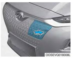
3. Push the charging door where the icon is located to open. The charging door opens only when the door is unlocked.
