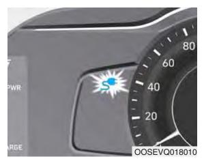
7. Check if the charging indicator light of the high voltage battery in the instrument cluster is turned ON. Charging is not done when the charging indicator lamp is OFF.
