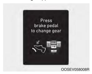
display, when the brake pedal is not depressed while shifting the gear.
