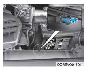
If the charging connector does not disconnect due to battery discharge and failure of the electric wires, open the hood and slightly pull the emergency cable. The charging connector will then disconnect.
