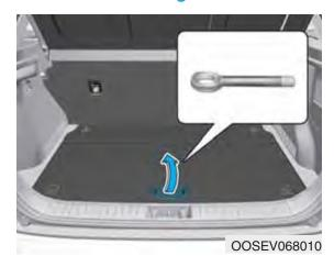
Open the tailgate and remove the towing hook from the tool case. The tool case is placed under the luggage tray.
