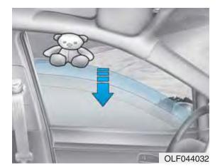
If a window senses any obstacle while it is closing automatically, it will stop and lower approximately 30 cm (12 inches) to allow the object to be cleared.
