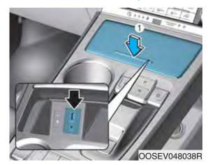
You can use an AUX port to connect audio devices and an USB port to plug in an USB and an iPod® port. To use the AUX, USB and iPod®, open the front console cover by slightly pressing the lower part of the cover (1).
