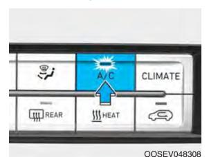
Push the A/C button to turn the air conditioning system on (indicator light will illuminate).
