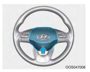
To sound the horn, press the area indicated by the horn symbol on your steering wheel. The horn will operate only when this area is pressed.
