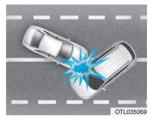
Air bags may not inflate if the vehicle collides with objects such as utility poles or trees, where the point of impact is concentrated and the collision energy is absorbed by the vehicle structure.
