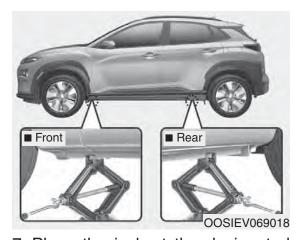
7. Place the jack at the designated jacking position under the frame closest to the tire you are changing. The jacking positions are plates welded to the frame with two notches. Never jack at any other position or part of the vehicle. It may damage the side seal molding.
