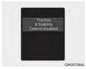
Press and hold the ESC OFF button continuously for more than 3 seconds. The ESC OFF indicator light and message "Traction & Stability Control disabled" illuminates and a warning chime sounds. In this state, both the traction control function of ESC and the brake control function of ESC are disabled.
