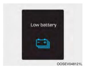
When the high voltage battery level reaches below approximately 8%, this warning message is displayed.
