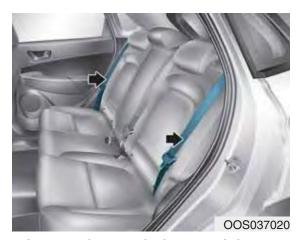
3.Locate the seatbelt toward the outboard position before folding down the seatback. If not, the seatbelt system may be interfered by the seatback.
