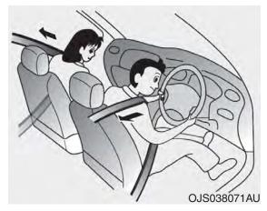
Your vehicle is equipped with Pretensioner Seat Belts (Retractor Pretensioner). The purpose of the pre-tensioner is to make sure the seat belts fit tightly against the occupant's body in certain frontal collisions. The pre-tensioner seat belts may be activated in crashes where the frontal collision is severe enough, together with the air bags.
