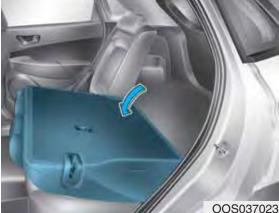
4.Remove the belt from the guide (1) and pull up the seatback folding lever (2), then fold the seat toward the front of the vehicle.
