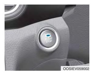
Whenever the front door is opened, the START/STOP button will illuminate and will go off 30 seconds after the door is closed.
