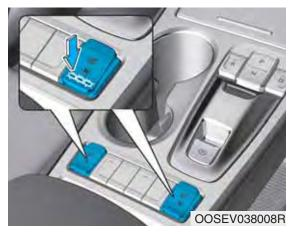
The air ventilation seats are provided to cool the front seats by blowing air through small vent holes on the surface of the seat cushions and seat-backs.
