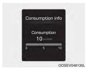
The trip computer mode displays information related to vehicle driving parameters including energy consumption, trip meter information and vehicle speed.
