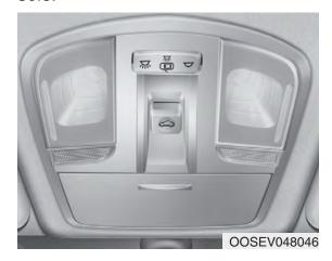
The sunroof can be opened, closed, or tilted when the START/STOP button is in the ON position.
