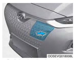
Push the charging door where the icon is located to open. The charging door opens only when the door is unlocked.
