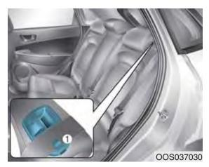
2. Make sure to insert the belt into the guide (1) and check that the seat belt is not twisted.
