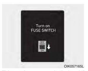
This warning message is displayed if the fuse switch located on the fuse box under the steering wheel is OFF. You should turn the fuse switch on.
