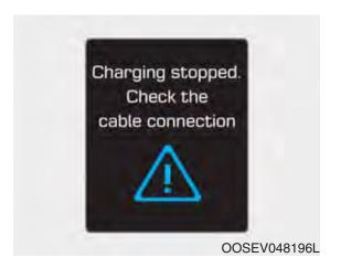
This warning message is displayed when charging is stopped because the charging connector is not correctly connected to the charging inlet
