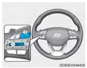
The steering wheel audio control switches are installed for your convenience.
