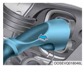
2.Hold the charging connector handle and pull it out.
