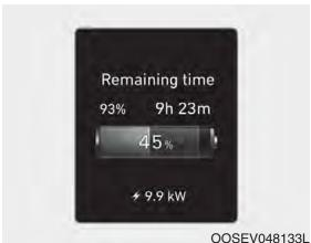
11. After charging has started, the estimated charging time is displayed on the instrument cluster for about 1 minute.
