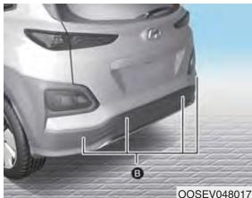
[A]: Front Sensor, [B]: Rear Sensor
