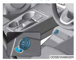
The power outlet is designed to provide power for mobile telephones or other devices designed to operate with vehicle electrical systems. The devices should draw less than 180 W(Watt) with the vehicle in the ready (\$\varpi\$) mode.
