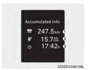
This display shows the accumulated trip distance (1), the average energy consumption (2), and the total driving time (3).
