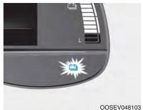
When there are 2 gauge bars (near the "L (Low)" area) on the SOC gauge, the warning lamp turns ON to alert you of the battery level.
