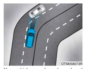
Your vehicle speed can be reduced due to a vehicle in the adjacent lane. Apply the accelerator pedal and select the appropriate speed. Check to be sure that the road conditions permit safe operation of the Smart Recuperation System.
