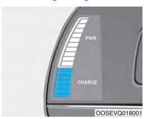
The Power/Charge Gauge shows the energy consumption rate of the vehicle and the charge/discharge status of the regenerative brakes.
