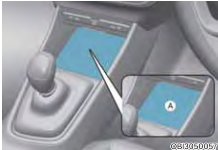
[A] : Charging pad
