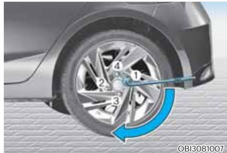
13. Use the wheel lug nut wrench to tighten the lug nuts in the order shown. Double-check each lug nut until they are tight. After changing tires, we recommend that an authorized HYUNDAI dealer tighten the lug nuts to their proper torque as soon as possible. **The wheel lug nut should be tightened to 11-13 kgf.m (79-94 lbf.ft).**
