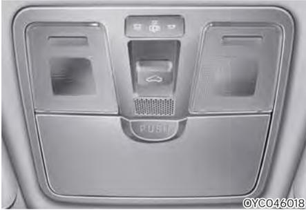
The sunroof can only be operated when the ignition switch or Engine Start/Stop button is in the ON or START position.
