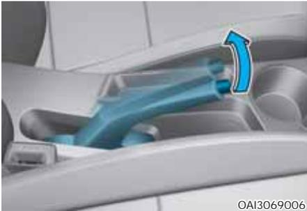
Check the stroke of the parking brake by counting the number of “clicks” heard while fully applying it from the released position.
