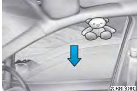
If a window senses any obstacle while it is closing automatically, it will stop and lower approximately 30 cm (12 inches) to allow the object to be cleared.
