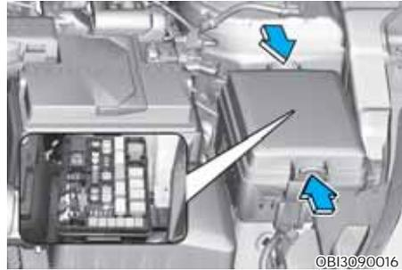
5. Pull the suspected fuse straight out. Use the removal tool provided in the engine compartment fuses panel.
