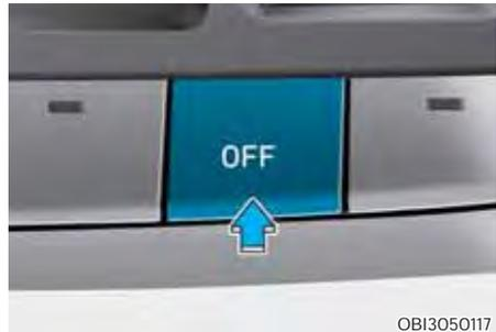
Push the OFF button to turn off the climate control system. You can still operate the mode and air intake buttons with the ignition switch in the ON position.
