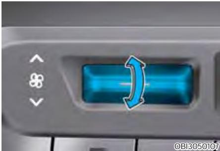
Push the switch to up to increase the fan speed and airflow. Push the switch to down to decrease fan speed and airflow.
