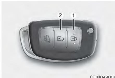
To lock the doors, press the Door Lock button (1) on the remote key.
