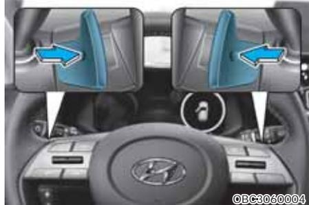
The paddle shifter is functional when the shift lever is in the D (Drive) position or the manual shift mode.
