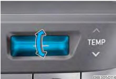
2. Push the temperature control switch to set the desired temperature. If the temperature is set to the lowest setting (Lo), the air conditioning system will operate continuously.
