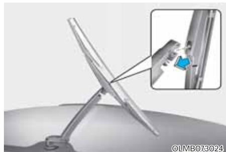
3. Install the new blade assembly by inserting the center part into the slot in the wiper arm until it clicks into place.
