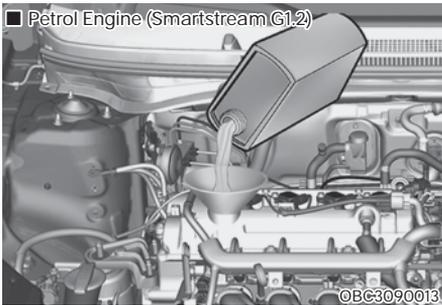
7. If the oil level is below L, add enough oil to bring the level to F (Full). **Do not overfill.**
