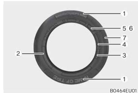
This information identifies and describes the fundamental characteristics of the tire and also provides the tire identification number (TIN) for safety standard certification. The TIN can be used to identify the tire in case of a recall.
