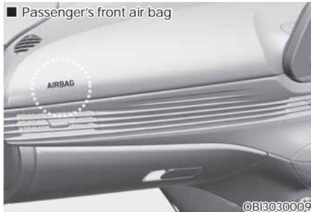
Your vehicle is equipped with a Supplemental Restraint (Air Bag) System and lap/shoulder belts at both the driver and passenger seating positions.
