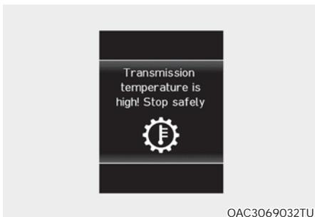
The following extreme cases may damage the clutch due to overheating while driving. Vehicle's own protection system sounds alarm and displays warning messages. Please shift into lower gear or stop the vehicle according to the instruction.
