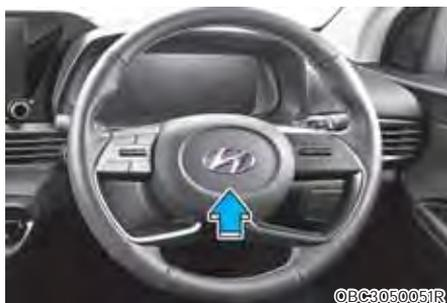
To sound the horn, press the area indicated by the horn symbol on your steering wheel (see illustration). The horn will operate only when this area is pressed.
