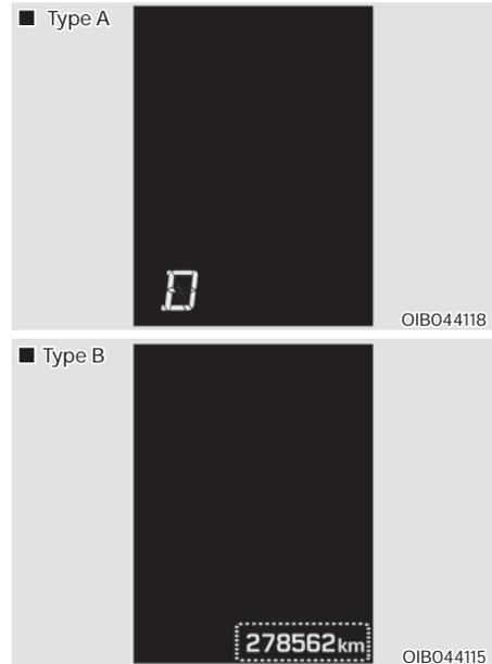
This indicator displays which dual clutch transmission shift lever is selected.
