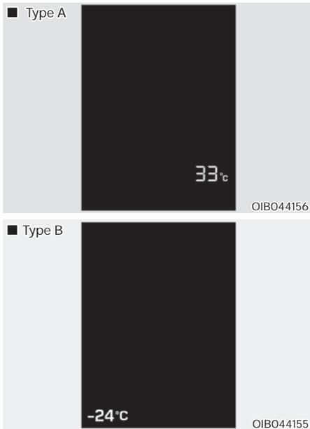
This gauge indicates the current outside air temperatures by 1°C (1°F).
