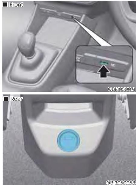
The USB charger is designed to recharge batteries of small size electrical devices using a USB cable.
