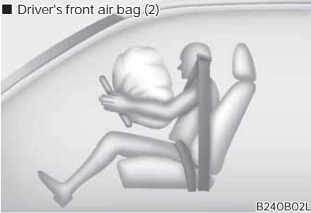
Upon deployment, tear seams molded directly into the pad covers will separate under pressure from the expansion of the air bags. Further opening of the covers then allows full inflation of the air bags.
