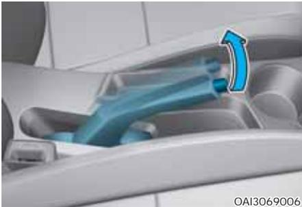
Always set the parking brake before leaving the vehicle, to apply:
