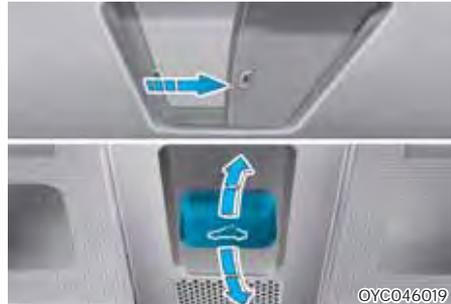
To open or close the sunroof (manual slide feature), push the sunroof control lever backward or forward to the first detent position.
