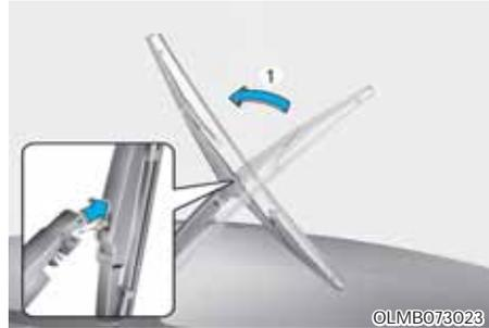
1. Raise the wiper arm and rotate the wiper blade assembly (1).
