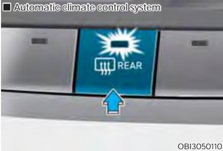
The defroster heats the window to remove frost, fog and thin ice from the interior and exterior of the rear window, while engine is running.
