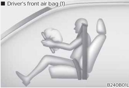
The air bag modules are located both in the center of the steering wheel and in the front passenger's panel above the glove box. When the SRSCM detects a sufficiently severe impact to the front of the vehicle, it will automatically deploy the front air bags.
