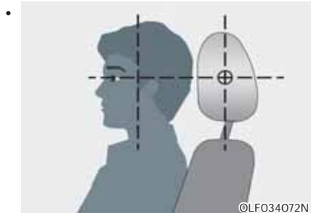
Adjust the headrests so the middle of the headrests is at the same height as the height of the top of the eyes.
