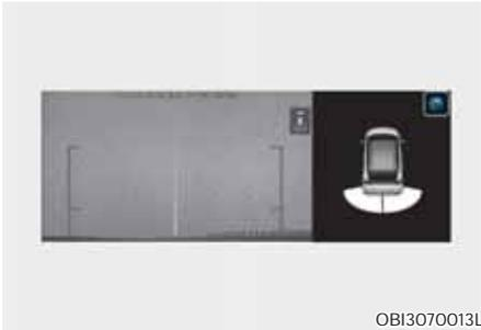
When you touch the
