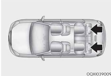
The rear seats are equipped with headrests in the outboard seating positions for the occupant's safety and comfort.
