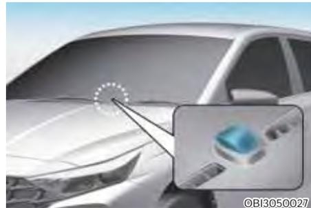
**Never place anything near the sensor located to ensure better control of the heating and cooling system.**
