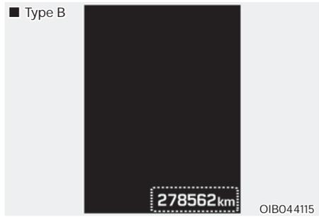
The odometer indicates the total distance that the vehicle has been driven and should be used to determine when periodic maintenance should be performed.
