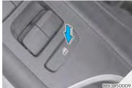
The driver can disable the power window switches on the rear passengers' doors by pressing the power window lock switch.
