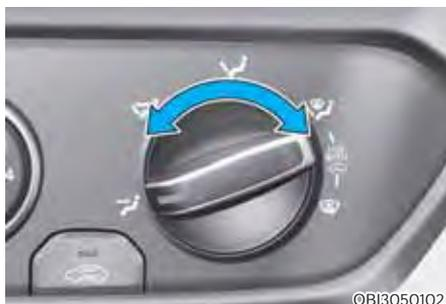
The mode selection knob controls the direction of the air flow through the ventilation system.
