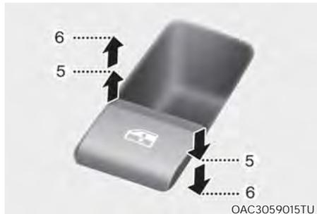
Pressing the power window switch momentarily to the second detent position (6) completely lowers the driver's window even when the switch is released. To stop the window at the desired position while the window is in operation, pull up and release the switch to the opposite direction of the window movement.
