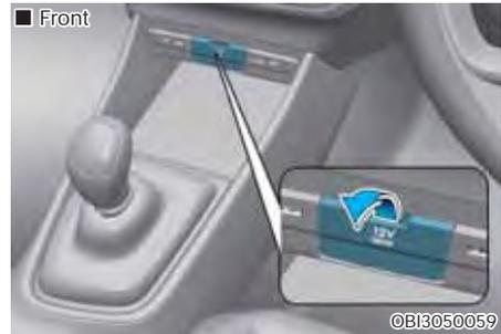
The power outlet is designed to provide power for mobile telephones or other devices designed to operate with vehicle electrical systems. The devices should draw less than 180W (Watt) with the engine running.
