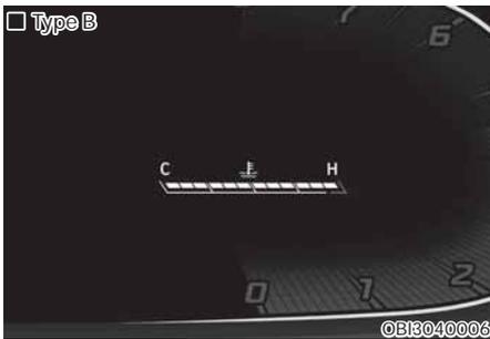
This gauge shows the temperature of the engine coolant when the ignition switch is in the ON position.
