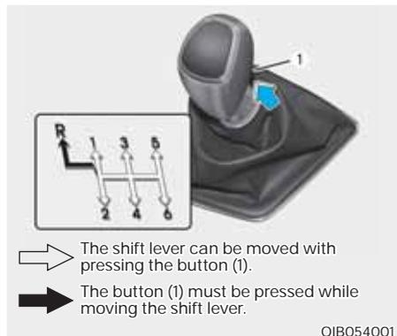
The intelligent manual transmission has 6 forward gears. This shift pattern is imprinted on the shift knob.
