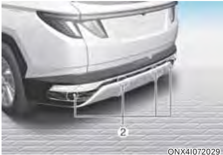
[2] : Rear ultrasonic sensors
