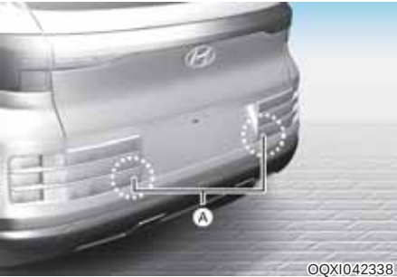
[A] : Rear ultrasonic sensors
