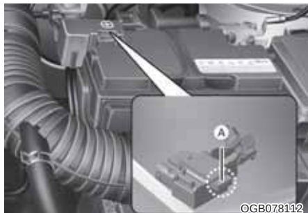
[A] : Battery sensor
