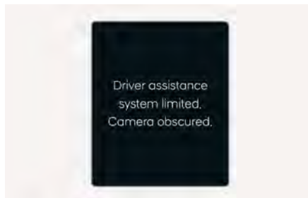
Front view camera obscured warning example
