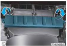
3. Remove the climate control air filter cover.
