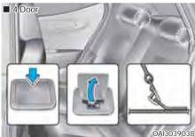
Top-tether anchorages for Child Restraint Systems are located on the floor of the luggage room (5 Door) or on the package tray (4 Door).
