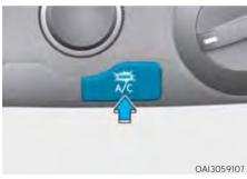
Press the A/C button to turn the air conditioning system on (indicator light will illuminate). Press the button again to turn the air conditioning system off.
