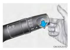
To flash the high beam headlights, pull the lever towards you, then release the lever. The high beams will remain ON as long as you hold the lever towards you.
