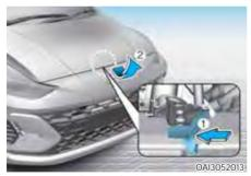
3. Go to the front of the vehicle, raise the hood slightly, push the secondary hood release lever up (1) inside of the hood center and lift the hood (2).
