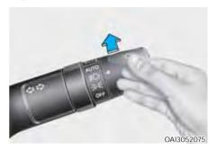
To turn on the high beam headlight, push the lever away from you. The lever will return to its original position.
