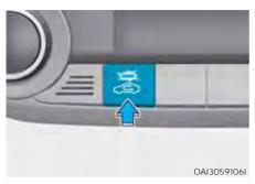
The air intake control button is used to select either Fresh mode (outside air) or Recirculation mode (cabin air).
