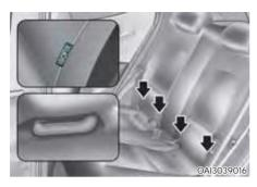
The ISOFIX anchorages symbols are located on the left and right rear seat cushions to identify the position of the ISOFIX anchorages in your vehicle (see arrows in illustration).
