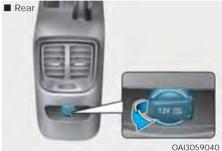
The power outlet is designed to provide power for mobile telephones or other devices designed to operate with vehicle electrical systems. The devices should draw less than 120 W (Watt) with the engine running.
