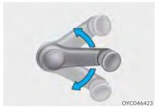
To raise or lower the window, turn the window regulator handle clockwise or counterclockwise in the right side. And the left side is opposite direction.
