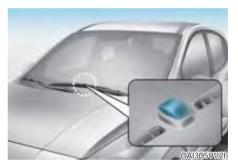
Never place anything near the sensor located to ensure better control of the heating and cooling system.
