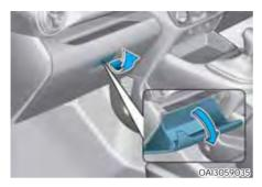
To open the glove box, pull the lever and the glove box will automatically open. Close the glove box after use.
