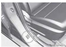
All specifications (sizes and pressures) can be found on a label attached to the driver's side center pillar.
