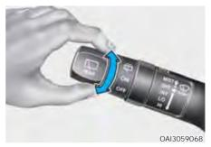
The rear window wiper and washer switches are located at the end of the wiper and washer switch lever.
