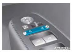
When pressing the (1) portion (1) of the switch, all vehicle doors will lock.
