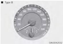
The speedometer indicates the speed of the vehicle and is calibrated in kilometers per hour (km/h).
