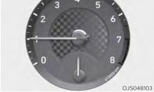
The tachometer indicates the approximate number of engine revolutions per minute (RPM).
