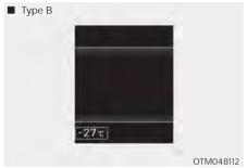
This gauge indicates the current outside air temperatures by 1 °C (1 °F).
