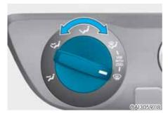
The mode selection knob controls the direction of the air flow through the ventilation system.
