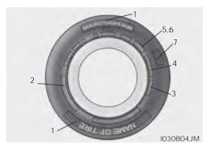
This information identifies and describes the fundamental characteristics of the tire and also provides the tire identification number (TIN) for safety standard certification. The TIN can be used to identify the tire in case of a recall.
