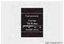
The trip computer mode displays information related to vehicle driving parameters including fuel economy, tripmeter information and vehicle speed.
