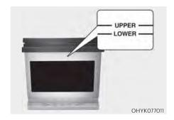
If your vehicle is equipped with a battery marked with LOWER (MIN) and UPPER (MAX) on the side, you should check the electrolyte level.
