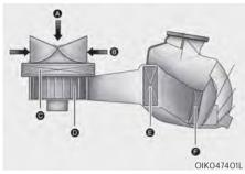
[A]: Outside air, [B]: Recirculated air [C]: Climate control air filter, [D]: Blower
