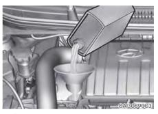
If the oil level is below L, add enough oil to bring the level to F (Full). Do not overfill.
