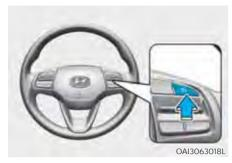
Pressing the Driving Assist button. The cruise indicator will go off.
