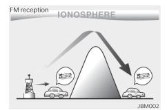
AM broadcasts can be received at greater distances than FM broadcasts. This is because AM radio waves are transmitted at low frequencies. These long distance, low frequency radio waves can follow the curvature of the earth rather than travelling straight. In addition, they curve around obstructions resulting in better signal coverage.
