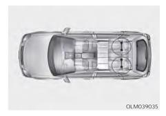
ISOFIX anchorages have been provided in the left and right outboard rear seating positions. Their locations are shown in the illustration. There are no ISOFIX anchorages provided for the center rear seating position.
