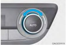
2. Turn the temperature control knob to set the desired temperature. If the temperature is set to the lowest setting (Lo), the air conditioning system will operate continuously. To turn the automatic operation off, select any button of the following:
