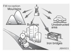
FM broadcasts are transmitted at high frequencies and do not bend to follow the earth's surface. Because of this, FM broadcasts generally begin to fade within short distances from the station. Also, FM signals are easily affected by buildings, mountains, and obstructions. This can lead to undesirable or unpleasant listening conditions which might lead you to believe a problem exists with your radio.
