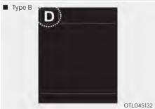
This indicator displays which Automated Manual Transmission shift lever is selected.
