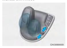
Whether the vehicle is stationary or in motion, Manual shift mode is selected by pushing the shift lever from the D (Drive) position into the manual gate (M). To return to D (Drive) range operation, push the shift lever back into the main gate.
