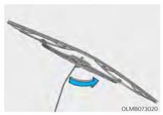
Raise the wiper arm and turn the wiper blade assembly to expose the plastic locking clip.
