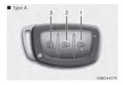
Your HYUNDAI uses a Smart Key, which you can use to lock or unlock a door (and trunk/tailgate) and even start the engine.
