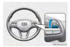
Push the RES+ switch up. If the vehicle speed is over 30 km/h (20 mph), the vehicle will resume the preset speed.
