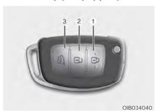
Your HYUNDAI uses a remote key, which you can use to lock or unlock a door (and trunk/tailgate) and even start the engine.
