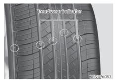
If the tire is worn evenly, a tread wear indicator will appear as a solid band across the tread. This shows there is less than 1.6 mm (1/16 inch) of tread left on the tire. Replace the tire when this happens.
