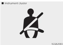
As a reminder to the front passenger, the front passenger's seat belt warning lights will illuminate for approximately 6 seconds each time you turn the ignition switch or Engine Start/Stop button ON regardless of belt fastening.
