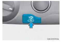
This button is used to select the outside (fresh) air position or recirculated air position.
