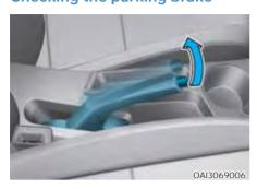
Check the stroke of the parking brake by counting the number of "clicks" heard while fully applying it from the released position.
