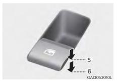
Pressing the power window switch momentarily to the second detent position (6) completely lowers the driver's window even when the switch is released. To stop the window at the desired position while the window is in operation, pull up and release the switch to the opposite direction of the window movement.
