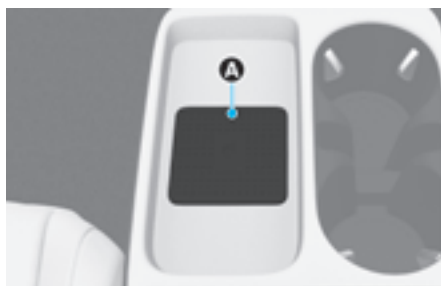
[A] Vehicle authentication pad (Wireless charging pad)
