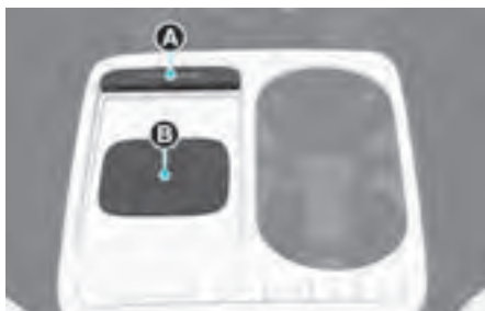
[A] Indicator light [B] Charging pad
