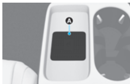
[A] Vehicle authentication pad (wireless charging pad)
