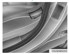
The vehicle certification label attached on the on the front passenger's side center pillar gives the vehicle identification number (VIN).
