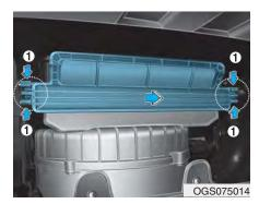
Remove the climate control air filter cover while pressing the lock
