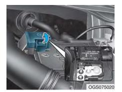
If an electrical system does not operate with no blown fuse in the engine room and inner fuse box, the main fuse inside the battery (+) cap may be blown.
