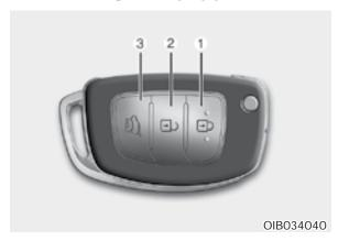
Your HYUNDAI uses a remote key, which you can use to lock or unlock a door (and tailgate) and even start the engine.
