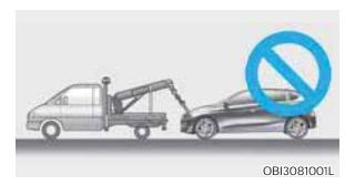
Do not tow the vehicle with the front wheels on the ground as this may cause damage to the vehicle and the Transmissions.
