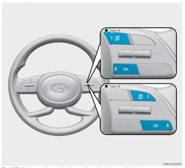
The LCD display modes can be changed by using the control buttons.
