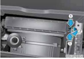
3. Remove the climate control air filter cover by pushing or pressing the clip (1) on right side.
