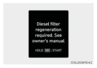
If the system still needs the self regeneration process after cancelling the operation, the warning message appears. (Diesel filter regeneration required.)
