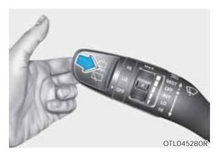
In the OFF position, pull the lever gently toward you to spray washer fluid on the windshield and to run the wipers 1-3 cycles. The spray and wiper operation will continue until you release the lever.
