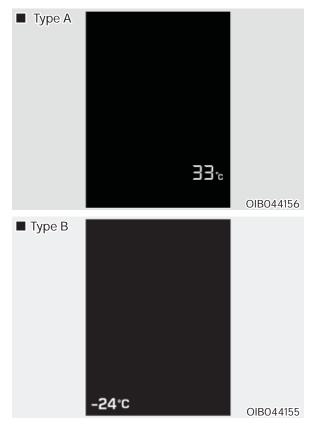
This gauge indicates the current outside air temperatures by 1°C (1°F).
