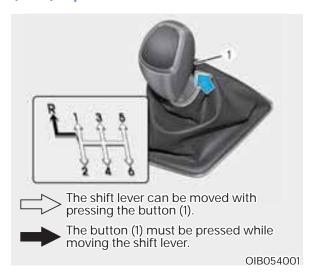
The Intelligent manual transmission (iMT) has 6 forward gears. This shift pattern is imprinted on the shift knob.
