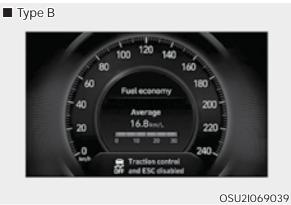
Press and hold the ESC OFF button continuously for more than 3 seconds. The ESC OFF indicator light and/or message "Traction control and ESC disabled" illuminates and a warning chime sounds. In this state, both the traction control function of ESC (engine management) and the brake control function of ESC (braking management) are disabled.
