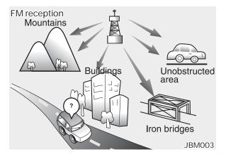
FM broadcasts are transmitted at high frequencies and do not bend to follow the earth's surface. Because of this, FM broadcasts generally begin to fade within short distances from the station. Also, FM signals are easily affected by buildings, mountains, and obstructions. This can lead to undesirable or unpleasant listening conditions which might lead you to believe a problem exists with your radio.
