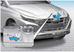
3. Go to the front of the vehicle, raise the hood slightly, push the secondary latch up (1) inside of the hood center and lift the hood (2).
