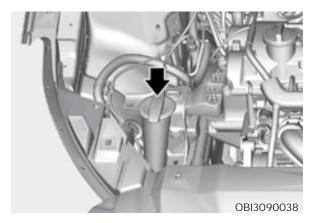
Check the fluid level in the washer fluid reservoir and add fluid if necessary. Plain water may be used if washer fluid is not available.
