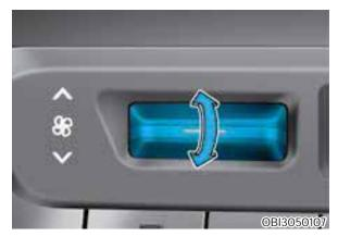
Push the switch to up to increase the fan speed and airflow. Push the switch to down to decrease fan speed and airflow.
