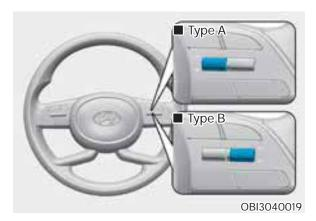
To change the trip mode, toggle the " $\land$ ,  $\checkmark$ " switch on the steering wheel.
