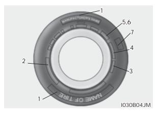
This information identifies and describes the fundamental characteristics of the tire and also provides the tire identification number (TIN) for safety standard certification. The TIN can be used to identify the tire in case of a recall.
