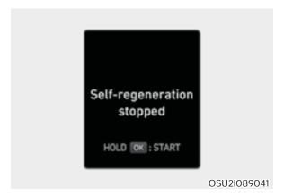
The self regeneration process stops if any of the self regeneration conditions is cancelled. If the self regeneration process is cancelled automatically, the system maintains "Self-regeneration stopped" message.
