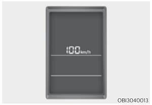
This message shows the speed of the vehicle (km/h, MPH).
