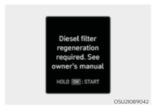
If the warning message "Diesel filter regeneration required, See owner's manual." appears on the LCD display, Self Regeneration is required.
