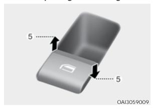
To open or close a window, press down or pull up the front portion of the corresponding switch to the first detent position (5).
