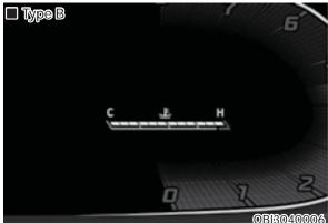
This gauge shows the temperature of the engine coolant when the ignition switch is in the ON position.
