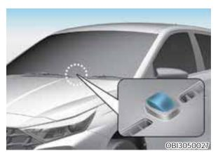
Never place anything near the sensor located to ensure better control of the heating and cooling system.
