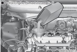
7. If the oil level is below L, add enough oil to bring the level to F (Full). **Do not overfill.**
