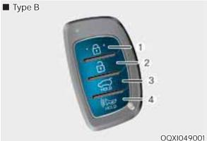
Your HYUNDAI uses a Smart Key, which you can use to lock or unlock a door (and tailgate) and even start the engine.
