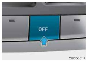
Push the OFF button to turn off the climate control system. You can still operate the mode and air intake buttons with the ignition switch in the ON position.
