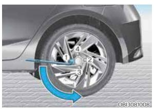
6. Loosen the wheel lug nuts counterclockwise one turn each in the order shown above, but do not remove any lug nuts until the tire has been raised off of the ground.
