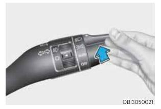
To turn on the high beam headlight, push the lever away from you. The lever will return to its original position.
