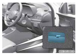
ALWAYS use the Floor Mat Anchors to attach the front floor mats to the vehicle. The anchors on the front floor carpet keep the floor mats from sliding forward.
