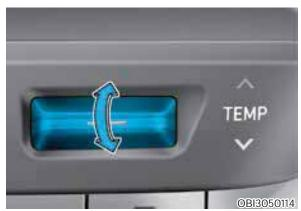
2. Push the temperature control switch to set the desired temperature. If the temperature is set to the lowest setting (Lo), the air conditioning system will operate continuously.
