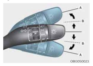
To signal a turn, push down on the lever for a right turn or up for a left turn in position (A). To signal a lane change, move the turn signal lever slightly and hold it in position (B). The lever will return to the OFF position when released or when the turn is completed.
