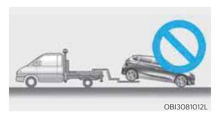
Do not tow with sling-type equipment. Use a wheel lift or flatbed equipment.
