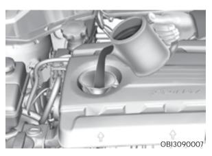
7. If the level is in the D range, add enough engine oil to bring the level up the range.
