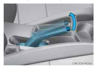
Check the stroke of the parking brake by counting the number of "clicks" heard while fully applying it from the released position.
