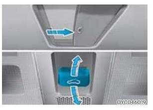
To open or close the sunroof (manual slide feature), push the sunroof control lever backward or forward to the first detent position.
