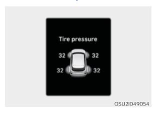
When the tire pressure monitoring system warning indicators are illuminated and a warning message displayed on the cluster LCD display, one or more of your tires is significantly under-inflated. The low tire pressure position telltale light will indicate which tire is significantly under-inflated by illuminating the corresponding position light.
