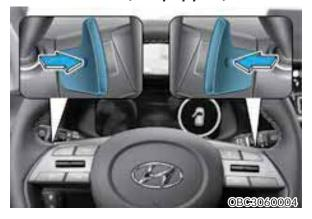
The paddle shifter is functional when the shift lever is in the D (Drive) position or the manual shift mode.
