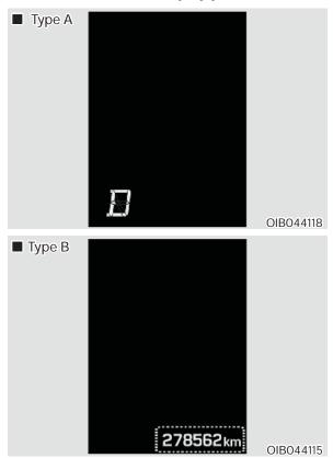
This indicator displays which continuously variable transmission shift lever is selected.
