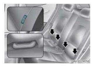
The ISOFIX anchorages symbols are located on the left and right rear seat cushions to identify the position of the ISOFIX anchorages in your vehicle (see arrows in illustration).
