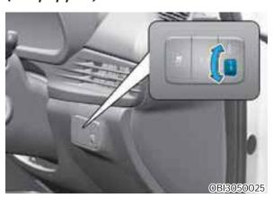
To adjust the headlight beam level according to the number of the passengers and loading weight in the luggage area, turn the beam leveling switch.
