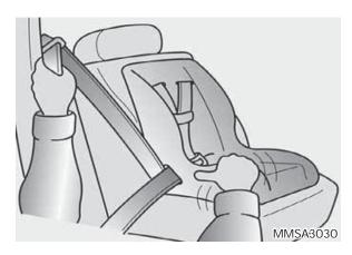
3. Buckle the seat belt and allow the seat belt to take up any slack. After installation of the child restraint system, try to move it in all directions to be sure the child restraint system is securely installed.
