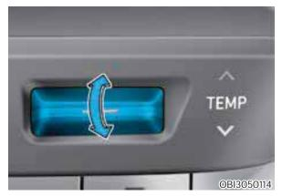
The temperature will increase by pushing the switch to up.
