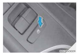
The driver can disable the power window switches on the rear passengers' doors by pressing the power window lock switch.
