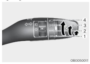
To operate the lights, turn the knob at the end of the control lever to one of the following positions:
