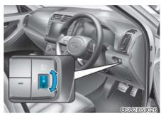
To adjust the headlight beam level according to the number of the passengers and loading weight in the luggage area, turn the beam leveling switch.
