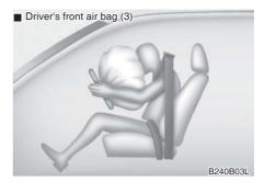
A fully inflated air bag, in combination with a properly worn seat belt, slows the driver's or the passenger's forward motion, reducing the risk of head and chest injury.
