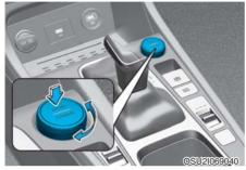
If you press the "DRIVE/TRACTION" mode button, the driving mode is changed from Driving control to Traction control. You can select SNOW, MUD or SAND mode by rotation the knob. If you press the "DRIVE/TRACTION" mode button again, the driving mode is changed from Traction Control to previous driving control.
