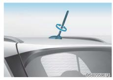
The antenna will receive AM, FM broadcast signals, etc. and transmit data. This antenna pole is removable. Rotate the antenna in a counterclockwise direction to remove it.
