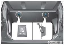
Top-tether anchorages for Child Restraint Systems are located on the floor of the luggage room.
