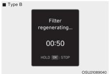
Operationg Self Regeneration Mode If the self regeneration mode starts, the message "Filter regenerationg..." and the remaining time appears. It takes around 30~60 minutes.
