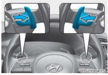
The paddle shifter is available when the shift lever is in the D (Drive) position or the manual shift mode.
