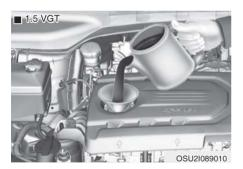
If it is near or at L, add enough oil to bring the level to F. Do not overfill.
