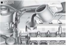
If it is near or at L (Low), add enough oil to bring the level to F (Full). **Do not overfill.**
