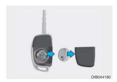
Battery Type: CR2032 To replace the battery:
