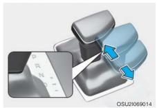
Whether the vehicle is stationary or in motion, manual shift mode is selected by pushing the shift lever from the D (Drive) position into the manual gate. To return to D (Drive) range operation, push the shift lever back into the main gate.
