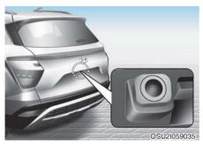
Rear View Monitor system will activate when the ignition switch is in the ON position and the shift lever is in the R (Reverse) position.
