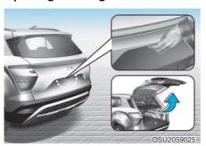
Make sure the shift lever is in P (Park, for Intelligent Variable Transmission/Dual Clutch Transmission/Automatic Transmission vehicle) position or first gear or R (Reverse, for Manual Transmission) position and set the parking brake.
