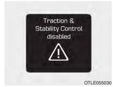
Press and hold the ESC OFF button continuously for more than 3 seconds. The ESC OFF indicator light and message (vehicles equipped with a supervision cluster) illuminates and a warning chime sounds. In this state, both the traction control function of ESC (engine management) and the brake control function of ESC (braking management) are disabled.
