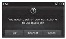
If Bluetooth® Wireless Technology devices are paired but none are currently connected, pressing the [PHONE] button or the [CALL] button on the steering wheel controls displays the following screen. Press the [Pair] to pair a new device or press the [Connect] to connect a previously paired device.
