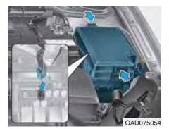
Before inspecting a fuse, you should turn OFF the engine as well as the other electric system switches. If a fuse is blown out, remove the blownout fuse and install a new fuse of the same capacity. Pay extreme caution not to damage the blown-out fuse while removing it.
