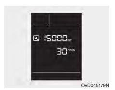
If the remaining mileage or time reaches 1,500 km (900 miles) or 30 days, the service symbol ( ) will blink for several seconds each time you set the ignition switch or Engine Start/Stop button to the ON position.
