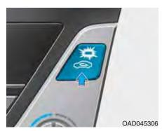
This is used to select outside (fresh) air position or recirculated air position. To change the air intake control position, press the control button.
