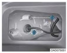
3.Loosen the assembly retaining nuts.
