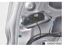
Disconnect the connector and then remove the nuts by turning the nuts counter clockwise.
