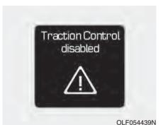
Press the ESC OFF button briefly. The ESC OFF indicator light and message (vehicles equipped with a supervision cluster) will illuminate. In this state, the traction control function of ESC (engine management) is disabled, but the brake control function of ESC (braking management) still operates.
