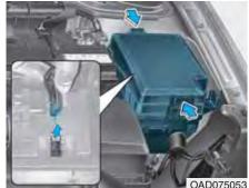
Before inspecting a fuse, you should turn OFF the engine as well as the other electric system switches. If a fuse is blown out, remove the blown-out fuse and install a new fuse of the same capacity by using the fuse puller, which is prepared inside the fuse box in the engine compartment. A new fuse may be prepared along with the fuse puller. However, if not, you may temporarily select/use a fuse of the other systems, which do not affect the vehicle operation, such as the audio system.
