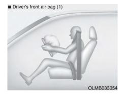
When the SRSCM detects a sufficiently severe impact to the front of the vehicle, it will automatically deploy the front air bags.
