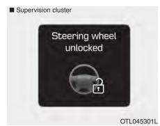
This warning message is displayed if the battery of the smart key is discharged while changing the Engine Start/Stop button while changing to the OFF position.
