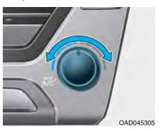
The temperature control knob allows you to control the temperature of the air flowing from the ventilation system. To change the air temperature in the passenger compartment, turn the knob to the right position for warm and hot air or left position for cooler air.
