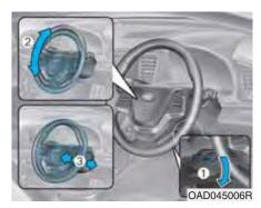
Pull down the lock-release lever (1) on the steering wheel column and adjust the steering wheel angle (2) and position (3, if equipped). Move the steering wheel, so it points toward your chest, not toward your face.
