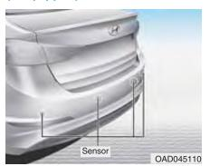
The Rear Parking Assist System assists the driver during reverse movement of the vehicle by chiming if any object is sensed within approximately 120 cm (50 in) behind the vehicle.
