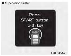
This warning message is displayed if the smart key is not detected when you press the Engine Start/Stop button.
