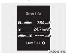
At the end of each driving cycle, the Driving Info message is displayed. This display shows the trip distance (1), the average fuel economy (2), and the remaining distance to empty (3).
