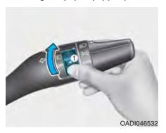
Fog lamps are used to provide improved visibility when visibility is poor due to fog, rain or snow, etc. Use the switch next to the headlamp switch to turn the fog lamps ON and OFF.
