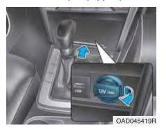
The power outlet is designed to provide power for mobile telephones or other devices designed to operate with vehicle electrical systems. The devices should draw less than 180 W(Watt) with the engine running.
