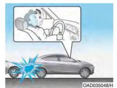
Front air bags are not designed to inflate in rear collisions, because occupants are moved backward by the force of the impact. In this case, inflated air bags would not provide any additional benefit.
