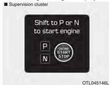
you press the Engine Start/Stop button while the warning message "Key not detected" is displayed.
