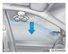
If a window senses any obstacle while it is closing automatically, it will stop and lower approximately 30 cm (12 inches) to allow the object to be cleared.
