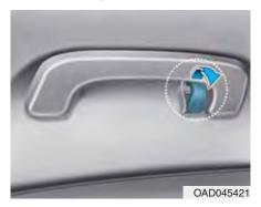
To hang items, pull the hanger down. These hangers are not designed to hold large or heavy items.
