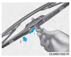
2. Press the clip and slide the blade assembly downward.
