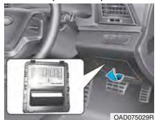
Inside the fuse/relay box covers, you can find the fuse/relay label describing fuse/relay name and capacity.
