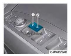
When pressing the  $(\frac{1}{1})$  portion (1) of the switch, all vehicle doors will lock.
