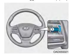
(RES+). If the vehicle speed is over 30 km/h, the vehicle will resume the preset speed.
