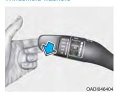
In the OFF (O) position, pull the lever gently toward you to spray washer fluid on the windshield and to run the wipers 1-3 cycles. The spray and wiper operation will continue until you release the lever. If the washer does not work, you may need to add washer fluid to the washer fluid reservoir.
