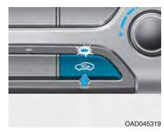
This is used to select the outside (fresh) air position or recirculated air position.
