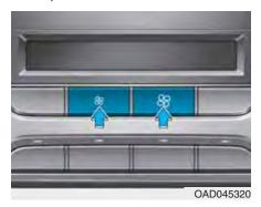
The fan speed can be set to the desired speed by pushing the fan speed control button.
