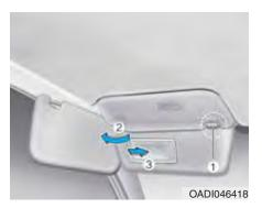
To use a sunvisor, pull it downward. To use a sunvisor for a side window, pull it downward, unsnap it from the bracket (1) and swing it to the side (2). To use the vanity mirror, pull down the sunvisor and slide the mirror cover (3).
