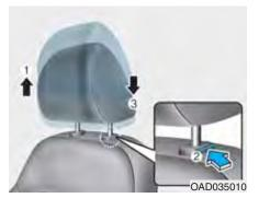
Adjusting the height up and down To raise the headrest:
