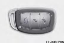
To lock the doors, press the button on the outside door handle while carrying the smart key with you or press the door lock button on the smart key. To unlock the doors, press the button on the outside door handle while carrying the smart key with you or press the door unlock button on the smart key.
