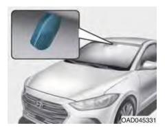
Auto defogging reduces the possibility of fogging up the inside of the windshield by automatically sensing the moisture of inside the windshield.
