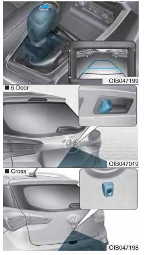
The Rear View Camera will activate when the engine is running and the shift lever is in the R (Reverse) position.
