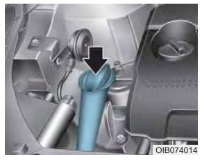
fluid reservoir and add fluid if necessary. Plain water may be used if washer fluid is not available.
