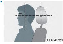
Adjust the headrests so the middle of the headrests is at the same height as the height of the top of the eyes.
