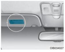
Air bag warning labels are attached to alert the driver and passengers of potential risks of the air bag system. Be sure to read all of the information about the air bags that are installed on your vehicle in this Owner's Manual.
