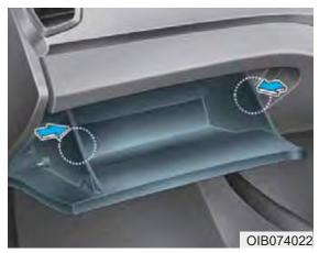
2. Push in both sides of the glove box as shown. This will ensure that the glove box stopper pins will get released from its holding location allowing the glove box to hang.
