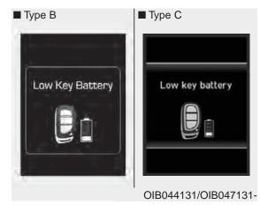
This warning message illuminates if the battery of the smart key is discharged when the Engine Start/Stop button is in the OFF position.
