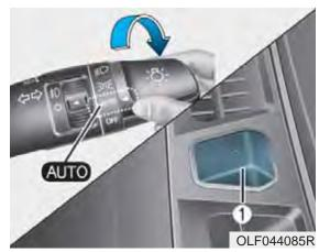
**AUTO light position (if equipped)** When the light switch is in the AUTO position, the parking (position) light and headlights will be turned ON or OFF automatically depending on the amount of light outside the vehicle.
