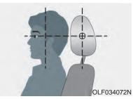
Adjust the headrests so the middle of the headrests is at the same height as the height of the top of the eyes.
