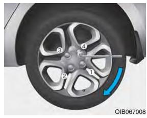
13. Use the wheel lug nut wrench to tighten the lug nuts in the order shown. Double-check each lug nut until they are tight. After changing tires, we recommend that an authorized HYUNDAI dealer tighten the lug nuts to their proper torque as soon as possible. The wheel lug nut should be tightened to 11~13 kgf.m (79~94 lbf.ft).
