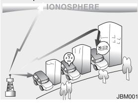
This can be due to factors, such as the distance from the radio station, closeness of other strong radio stations or the presence of buildings, bridges or other large obstructions in the area.
