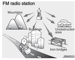
FM broadcasts are transmitted at high frequencies and do not bend to follow the earth's surface. Because of this, FM broadcasts generally begin to fade within short distances from the station. Also, FM signals are easily affected by buildings, mountains, and obstructions. This can lead to undesirable or unpleasant listening conditions which might lead you to believe a problem exists with your radio. The following conditions are normal and do not indicate radio trouble:
