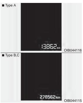
The odometer indicates the total distance that the vehicle has been driven and should be used to determine when periodic maintenance should be performed.
