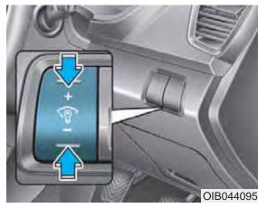
The brightness of the instrument panel illumination changes by pressing the upper or lower part of the switch when the ignition switch is in the ON position and when the parking lights are turned on.
