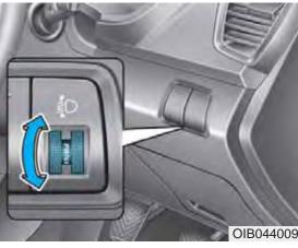
To adjust the headlight beam level according to the number of the passengers and loading weight in the luggage area, turn the beam leveling switch. The higher the number of the switch position, the lower the headlight beam level. Always keep the headlight beam at the proper leveling position, or headlights may dazzle other road users.
