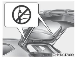
Do not hold the part (gas lifter) that supports the tailgate. Be aware that the deformation of the part may cause vehicle damage and a risk of safety accident. Emergency tailgate safety release
