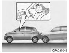
• Front air bags are not designed to inflate in rear collisions, because occupants are moved backward by the force of the impact. In this case, inflated air bags would not be able to provide any additional benefit.
