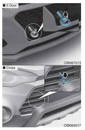
1.Open the trunk, and remove the towing hook from the tool case.
