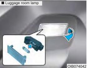
1. Using a flat-blade screwdriver, gently pry the lens from the interior light housing.
