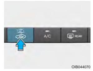
This button is used to select the outside (fresh) air position or recirculated air position. If the air flow rate suddenly decreases, we recommend the system be checked at an authorized HYUNDAI dealer.
