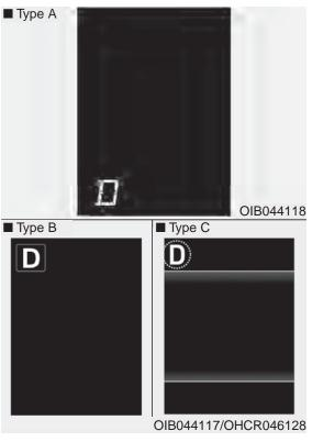
This indicator displays which Continuously Variable Transaxle shift lever is selected.
