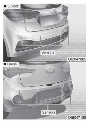
The Parking Distance Warning (Reverse) System assists the driver during reverse movement of the vehicle by chiming if any object is sensed within the distance of about 120 cm (47 in.) behind the vehicle. This is a supplemental system that senses objects within the range and location of the sensors, it cannot detect objects in other areas where sensors are not installed.
