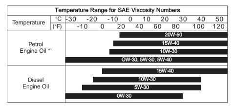
\*1: For better fuel economy, it is recommended to use the engine oil of a viscosity grade SAE 5W-30 (ACEA A5/B5). However, if the engine oil is not available in your country, select the proper engine oil using the engine oil viscosity chart.
