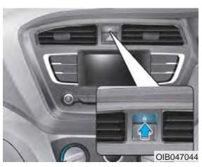
When you press the door lock/unlock switch, all vehicle doors will lock and the indicator light on the switch will illuminate for approximately 60 seconds (If the key is in the ignition switch, the indicator light on the switch will continuously illuminate).
