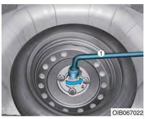
If it is hard to loosen the tire holddown wing bolt by hand, you can loosen it easily using the wheel lug nut wrench.
