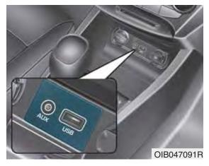
You can use an AUX port to connect audio devices and an USB port to plug in an USB or an iPod<sup>®</sup>.
