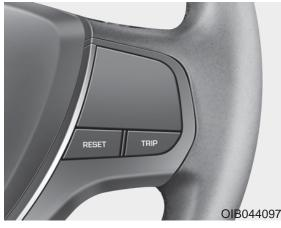
To change the trip mode, press the TRIP button on the steering wheel.
