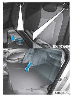
3. Pull up both sides of the seatback lever and fold the seatback toward the front of the vehicle.
