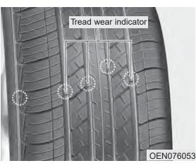
If the tire is worn evenly, a tread wear indicator will appear as a solid band across the tread. This shows there is less than 1.6 mm (1/16 inch) of tread left on the tire. Replace the tire when this happens.
