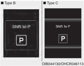
if you try to turn off the engine without the shift lever in P (Park) position.
