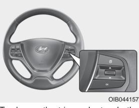
To change the trip mode, toggle the " $\land$ ,  $\checkmark$ " switch on the steering wheel.
