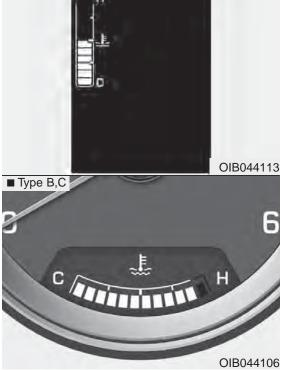
Engine Coolant Temperature
