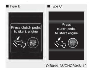
This warning message illuminates if the Engine Start/Stop button is in the ACC position twice by pressing the button repeatedly without depressing the clutch pedal.
