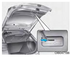
Your vehicle is equipped with the emergency tailgate safety release lever located on the bottom of the tailgate. When someone is inadvertently locked in the luggage compartment, the tailgate can be opened by doing as follows:
