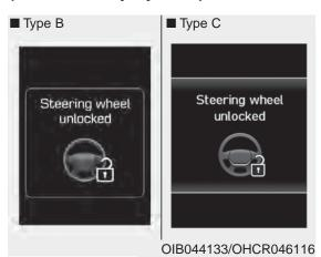
This warning message illuminates if the steering wheel does not lock when the Engine Start/Stop button is in the OFF position.
