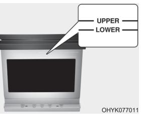
If your vehicle is equipped with a battery marked with LOWER (MIN) and UPPER (MAX) on the side, you should check the electrolyte level.
