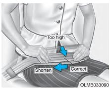
With a 2-point static type seat belt, the length must be adjusted manually so it fits snugly around your body. Fasten the belt and pull on the loose end to tighten. The belt should be placed as low as possible on your hips, not on your waist. If the belt is too high, it could increase the possibility of your being injured in an accident.
