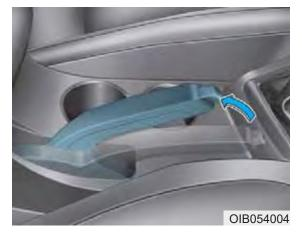
Check the stroke of the parking brake by counting the number of "clicks" heard while fully applying it from the released position. Also, the parking brake alone should securely hold the vehicle on a fairly steep grade. If the stroke is more or less than specified, we recommend that the system be inspected by an authorized HYUNDAI dealer.
