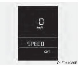
The digital speedometer is displayed when "SPEED" sets "ON" in the cluster.
