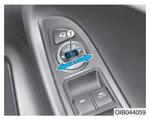
**Electric type (if equipped)** Adjusting the rearview mirrors:
