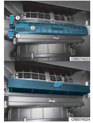
3. Remove the climate control air filter cover by pushing or pressing the clip (1) on left side.
