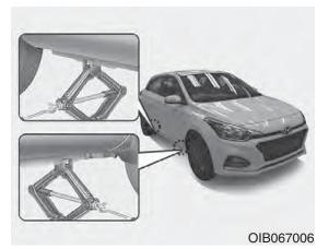
7.Place the jack at the designated jacking position under the frame closest to the tire you are changing. The jacking positions are plates welded to the frame with two tabs and a raised dot. Never jack any other position or part of the vehicle.
