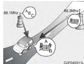
Multi-Path Cancellation - Radio signals being received from several directions can cause distortion or fluttering. This can be caused by a direct and reflected signal from the same station, or by signals from two stations with close frequencies. If this occurs, select another station until the condition has passed.
