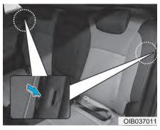
2. Insert the rear lap/shoulder belt plate into the holder on the side trim. It will prevent the lap/shoulder belt from interfering with the seatback when folding.
