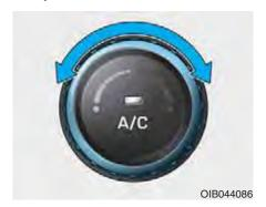
The temperature will increase to the maximum (HI) by turning the knob to the right.
