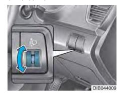
To adjust the headlight beam level according to the number of the passengers and loading weight in the luggage area, turn the beam leveling switch.
