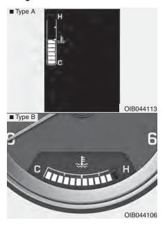
This gauge shows the temperature of the engine coolant when the ignition switch is in the ON position.
