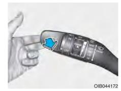
In the OFF position, pull the lever gently toward you to spray washer fluid on the windshield and to run the wipers 1-3 cycles. Use this function when the windshield is dirty. The spray and wiper operation will continue until you release the lever.
