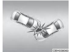
In a slant or angled collision, the force of impact may direct the occupants in a direction where the air bags would not be able to provide any additional benefit, and thus the sensors may not deploy any air bags.
