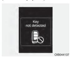
This warning message illuminates if the smart key is not detected when you press the Engine Start/Stop button.
