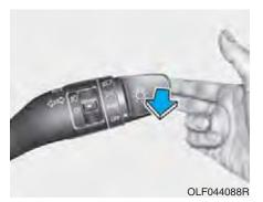
To flash the high beam headlights, pull the lever towards you, then release the lever. The high beams will remain ON as long as you hold the lever towards you.
