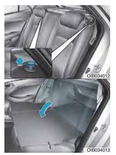
Pull up both sides of the seatback lever and fold the seatback toward the front of the vehicle.
