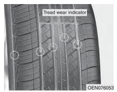
If the tire is worn evenly, a tread wear indicator will appear as a solid band across the tread. This shows there is less than 1.6 mm (1/16 inch) of tread left on the tire. Replace the tire when this happens.
