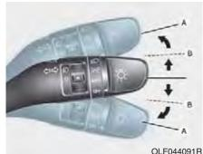
To signal a turn, push down on the lever for a right turn or up for a left turn in position (A). To signal a lane change, move the turn signal lever slightly and hold it in position (B). The lever will return to the OFF position when released or when the turn is completed.
