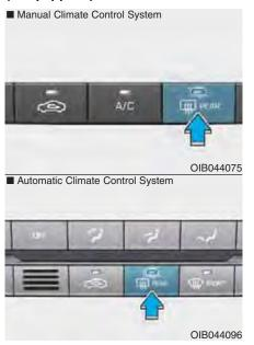
The defroster heats the window to remove frost, fog and thin ice from the interior and exterior of the rear window, while engine is running.
