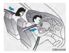
Your vehicle is equipped with driver's and front passenger's pre-tensioner seat belts. The purpose of the pre-tensioner is to make sure that the seat belts fit tightly against the occupant's body in certain frontal collisions. The pre-tensioner seat belts may be activated in crashes where the frontal collision is severe enough.
