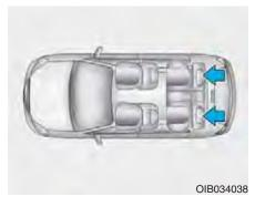
The rear seats are equipped with headrests in all the seating positions for the occupant's safety and comfort.
