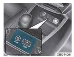
You can use an AUX port to connect audio devices and an USB port to plug in an USB and also in an iPod<sup>®</sup> port.
