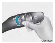
Fog lights are used to provide improved visibility when visibility is poor due to fog, rain or snow, etc.
