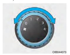
Turn the knob to the right to increase the fan speed and airflow. Turn the knob to the left to decrease fan speed and airflow.
