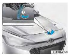
3. Go to the front of the vehicle, raise the hood slightly, push the secondary latch up (1) inside of the hood center and lift the hood (2).
