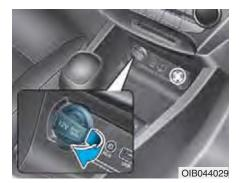
The power outlet is designed to provide power for mobile telephones or other devices designed to operate with vehicle electrical systems. The devices should draw less than 180W (Watt) with the engine running.
