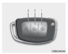
Your HYUNDAI uses a remote key, which you can use to lock or unlock a door (and tailgate) and even start the engine.
