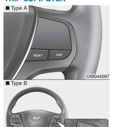
The trip computer is a microcomputer-controlled driver information system that displays information related to driving, when the ignition switch is in the ON position. All stored driving information (except odometer) resets if the battery is disconnected.
