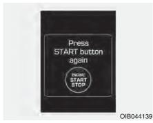
This warning message illuminates if you cannot operate the Engine Start/Stop button when there is a problem with the Engine Start/Stop button system.
