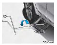
8. Insert the jack handle into the jack and turn it clockwise, raising the vehicle until the tire clears the ground. Make sure the vehicle is stable on the jack.
