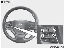
The steering wheel audio control button is installed to promote safe driving.
