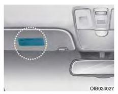
Air bag warning labels are attached to alert the driver and passengers of potential risks of the air bag system. Be sure to read all of the information about the air bags that are installed on your vehicle in this Owner's Manual.
