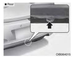
If towing service is not available in an emergency, your vehicle may be temporarily towed using a cable or chain secured to the emergency towing hook at the front (or rear) of the vehicle.
