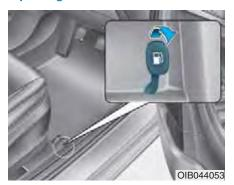
The fuel filler door must be opened from inside the vehicle by pulling up the fuel filler door opener.
