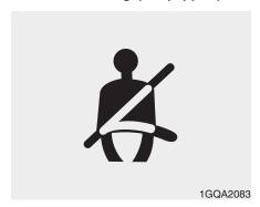
As a reminder to the driver, the seat belt warning light will blink for approximately 6 seconds each time you turn the ignition switch ON regardless of belt fastening.
