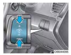
The brightness of the instrument panel illumination changes by pressing the upper or lower part of the switch when the ignition switch is in the ON position and when the parking lights are turned on.
