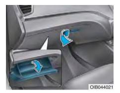
To open the glove box, pull the lever and the glove box will automatically open. Close the glove box after use.
