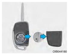
Battery Type: CR2032 To replace the battery:
