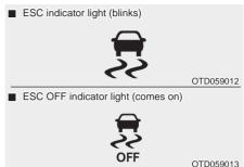
When the ignition switch is in the ON position, the ESC indicator light illuminates, then goes off if the ESC system is operating normally.
