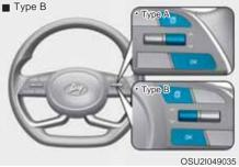
To change the trip mode, toggle the "\( \sim, \subseteq" \) switch on the steering wheel
