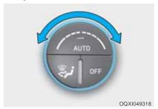
The temperature will increase to the maximum (HI) by turning the knob to the right.
