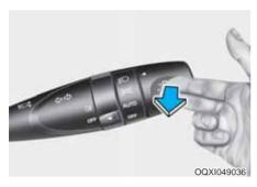
To flash the high beam headlights, pull the lever towards you, then release the lever. The high beams will remain ON as long as you hold the lever towards you.
