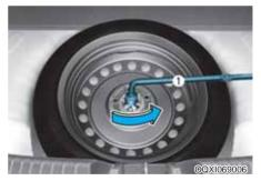
If it is hard to loosen the tire holddown wing bolt by hand, you can loosen it easily using the wheel lug nut wrench.
