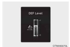
This mode dispalys the approximate amount of remaining urea solution inside the urea solution tank.
