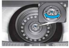
Turn the winged hold down bolt counterclockwise to remove the spare tire. Store the spare tire in the same compartment by turning the winged hold down bolt clockwise.
