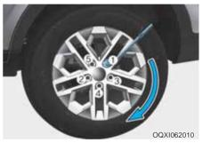
13. Use the wheel lug nut wrench to tighten the lug nuts in the order shown. Double-check each lug nut until they are tight. After changing tires, we recommend that an authorized HYUNDAI dealer tighten the lug nuts to their proper torque as soon as possible. The wheel lug nut should be tightened to 11~13 kgf.m (79~94 lbf.ft).
