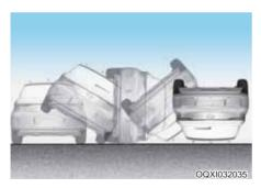
Air bags do not inflate in rollover accidents because vehicle can not detect rollover accident.
