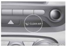
When the ignition switch is in the ON position, the clean air function turns on automatically.
