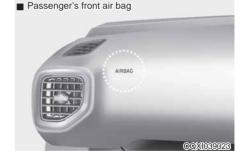
Your vehicle is equipped with a Supplemental Restraint (Air Bag) System and lap/shoulder belts at both the driver and passenger seating positions. The indications of the system's presence are the letters "AIR BAG" engraved on the air bag pad cover in the steering wheel and the passenger's side front panel pad above the glove box.
