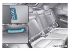
The ISOFIX anchorages symbols are located on the left and right rear seat to identify the position of the ISOFIX anchorages in your vehicle (see arrows in illustration).
