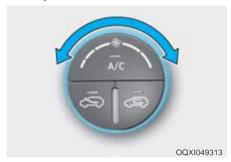
Turn the knob to the right increase the fan speed and air flow. Turn the knob to the left to decrease fan speed and air flow
