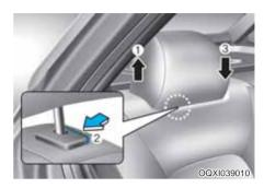
Adjusting the height up and down (if equipped)
