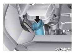
Check the fluid level in the washer fluid reservoir and add fluid if necessary. Plain water may be used if washer fluid is not available.
