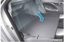
4. Pull up both sides of the seatback lever and fold the seatback toward the front of the vehicle.
