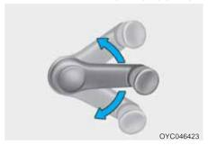
To raise or lower the window, turn the window regulator handle clockwise or counterclockwise in right side. And left side is opposite direction.
