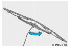
1. Raise the wiper arm and turn the wiper blade assembly to expose the plastic locking clip.
