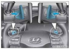
The paddle shifter is available when the shift lever is in the D (Drive) position.
