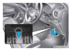
Your vehicle is equipped with the memory fuse to prevent battery discharge if your vehicle is parked without being operated for prolonged periods. Use the following procedures before parking the vehicle for prolonged periods.
