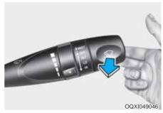
In the OFF position, pull the lever gently toward you to spray washer fluid on the windshield and to run the wipers 1-3 cycles. Use this function when the windshield is dirty. The spray and wiper operation will continue until you release the lever.
