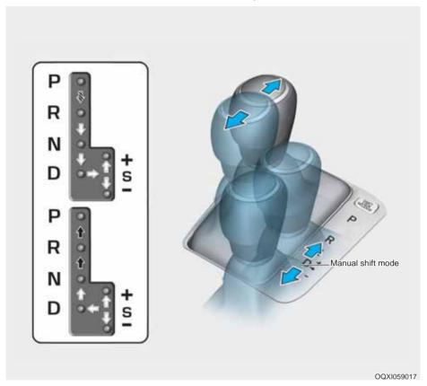
Depress the brake pedal and press the shift button while moving the shift lever.
