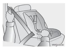
Buckle the seat belt and allow the seat belt to take up any slack. After installation of the child restraint system, try to move it in all directions to be sure the child restraint system is securely installed.
