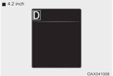
This indicator displays which duel clutch transmission shift lever is selected.
