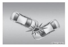
In a slant or angled collision, the force of impact may direct the occupants in a direction where the air bags would not be able to provide any additional benefit, and thus the sensors may not deploy any air bags.
