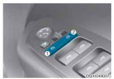
When pressing the  $( \frac{1}{1} )$  portion (1) of the switch, all vehicle doors will lock.
