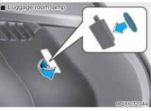
Using a flat-blade screwdriver, gently pry the lens from the interior light housing.
