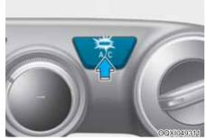
Press the A/C button to turn the air conditioning system on (indicator light will illuminate). Press the button again to turn the air conditioning system off.
