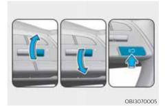
Operate the +, - switch or **II** button. If you push the + switch up or - switch down, the vehicle speed will be set to the current speed on the cluster.
