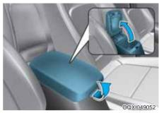
To open the center console storage, pull up the lever.
