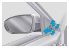
Manual type (if equipped) To adjust an outside mirror, move the control lever
