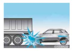
Just before impact, drivers often brake heavily. Such heavy braking lowers the front portion of the vehicle causing it to "ride" under a vehicle with a higher ground clearance. Air bags may not inflate in this "under-ride" situation because deceleration forces that are detected by sensor may be significantly reduced by such "under-ride" collisions.
