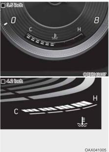
This gauge shows the temperature of the engine coolant when the ignition switch is in the ON position.
