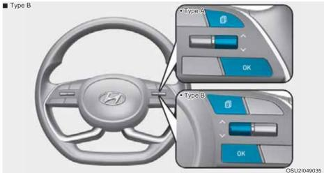
The LCD display modes can be changed by using the control buttons.
