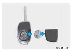
Battery Type: CR2032 To replace the battery:
