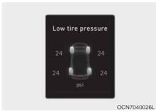
This warning message is displays if the tire pressure is low. The corresponding tire on the vehicle will be illuminated.
