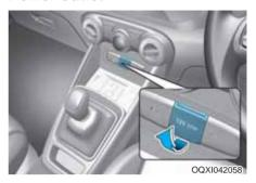
The power outlet is designed to provide power for mobile telephones or other devices designed to operate with vehicle electrical systems. The devices should draw less than 120W (Watt) with the engine running.
