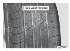
If the tire is worn evenly, a tread wear indicator will appear as a solid band across the tread. This shows there is less than 1.6 mm (1/16 inch) of tread left on the tire. Replace the tire when this happens.
