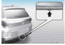
If towing service is not available in an emergency, your vehicle may be temporarily towed using a cable or chain secured to the emergency towing hook at the front (or rear) of the vehicle.
