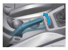
Check the stroke of the parking brake by counting the number of "clicks" heard while fully applying it from the released position. Also, the parking brake alone should securely hold the vehicle on a fairly steep grade. If the stroke is more or less than specified, we recommend that the system be inspected by an authorized HYUNDAI dealer.
