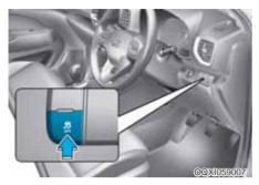
The Electronic Stability Control (ESC) system helps to stabilize the vehicle during cornering maneuvers.
