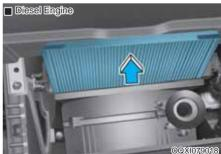
3. Remove the climate control air filter cover by pushing or pressing the clip (1) on left side.
