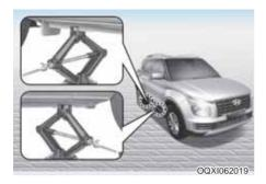
7. Place the jack at the designated jacking position under the frame closest to the tire you are changing. The jacking positions are plates welded to the frame with two tabs and a raised dot. Never jack any other position or part of the vehicle.
