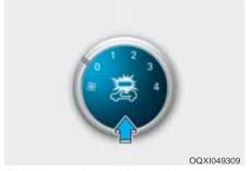
This button is used to select the outside (fresh) air position or recirculated air position.
