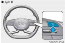
Press the Driving Assist button to turn Cruise Control off. The Cruise indicator will go off.
