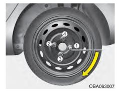
13. Use the wheel lug nut wrench to tighten the lug nuts in the order shown. Double-check each lug nut until they are tight. After changing tires, we recommend that an authorized HYUNDAI dealer tighten the lug nuts to their proper torque as soon as possible. The wheel lug nut should be tightened to 11~13 kg.m (79~94 lb.ft).
