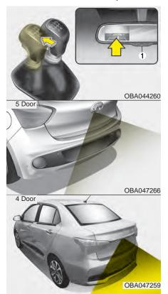
The rearview camera will activate when the back-up light is ON with the ignition switch ON and the shift lever in the R (Reverse) position.
