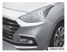
Headlight, position light, turn signal light, and front fog light bulb replacement
