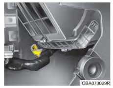
Remove the climate control air filter cover.
