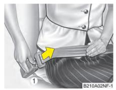
To release the seat belt: Press the release button (1) on the buckle and remove the metal tab from the buckle.
