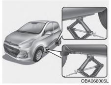
7. Place the jack at the designated jacking position under the frame closest to the tire you are changing. The jacking positions are plates welded to the frame with two tabs and a raised dot. Never jack any other position or part of the vehicle.
