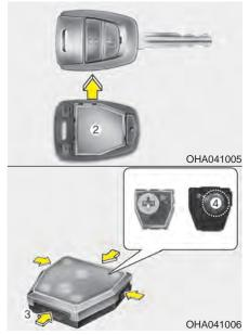
3. Open the inner remote key cover (2) by removing the hook from the slots (3).
