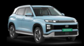
2 Battery packs: 42 kWh & 51,4 kWh
