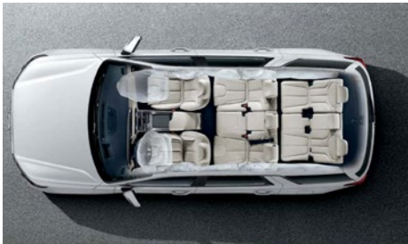
Multi-collision airbag system
